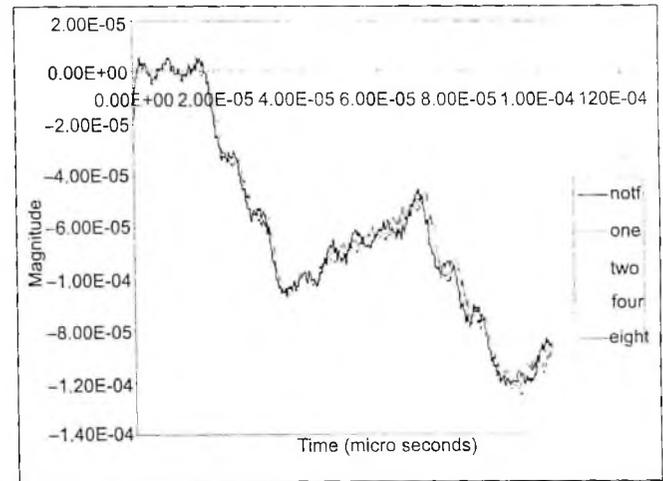
FIG. 2. NEUTRAL CURRENTS FOR VARIOUS TURN FAULT CONDITIONS IN SECTION BETWEEN NODE 17-18
