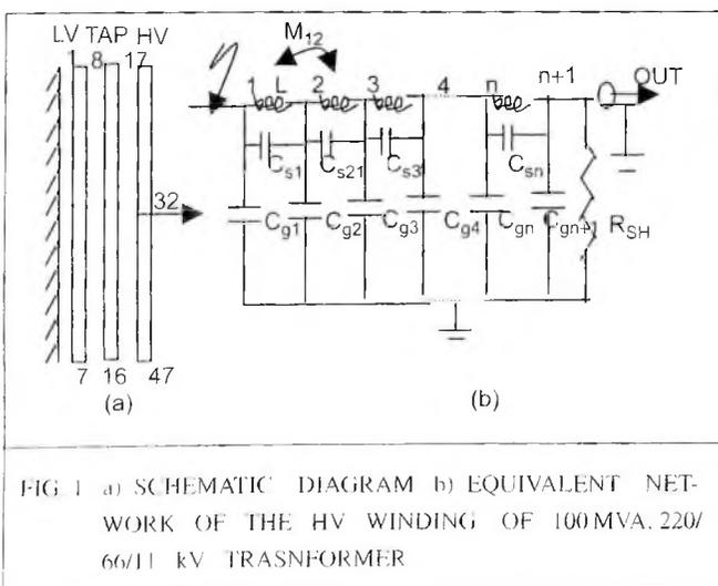
FIG 1 a) SCHEMATIC DIAGRAM b) EQUIVALENT NETWORK OF THE HV WINDING OF 100 MVA, 220/66/11 kV TRANSFORMER
