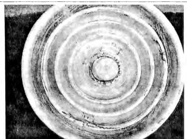
FIG. 8. SAMPLE AGED IN 25 mS/m. SHOWING CARBONIZATION OF THE OUTER MOST UNDER RIB
