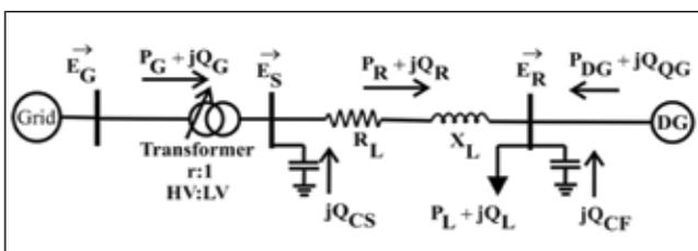
FIG.1 SIMPLIFIED SINGLE LINE DIAGRAM FOR PROBLEM FORMULATION
