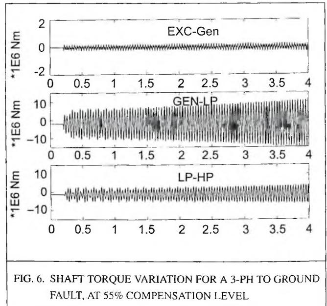
FIG. 6. SHAFT TORQUE VARIATION FOR A 3-PH TO GROUND FAULT, AT 55% COMPENSATION LEVEL
