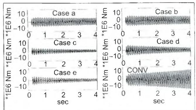
FIG. 8. GEN-LP SHAFT TRANSIENT TORQUE FOR A 3-PH TO GROUND FAULT FOR CASES A-E. CONV- FOR 55% COMPENSATION IN ALL PHASES
