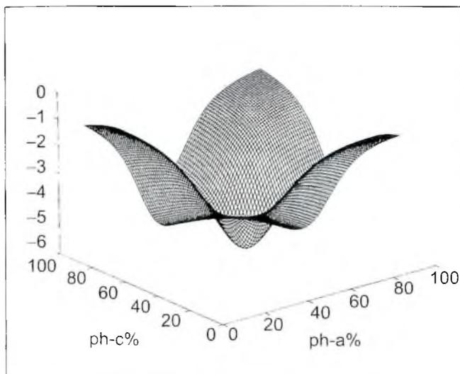
FIG 7. VARIATION OF  $T_D$  AT 24.6 HZ FOR 55% IN PHASE-B AND DIFFERENT COMPENSATION LEVELS IN PHASES A & C
