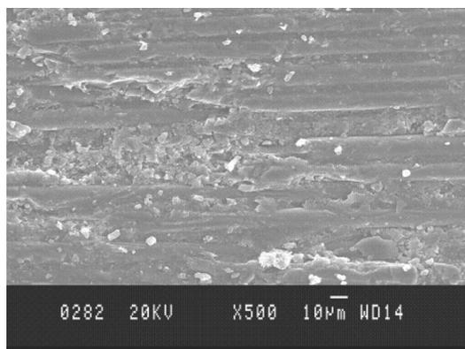
FIGS. 4 WORN SURFACE FEATURE OF C-V COMPOSITE UNDER QUARTZ ABRASIVE; (C) 270 M, AND (D) 1080 M
