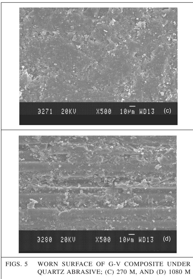
It is summarized that the use of C-V composite is desirable for the tribological applications in view of lower abrasion loss obtained due to the less debris formation and fiber breakage. Also, it is seen that the bonding between the fiber and the vinyl ester matrix seems to be favorable as the fibers not getting dislodged.
