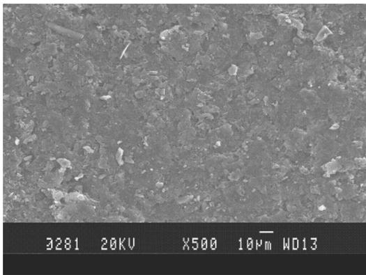
FIGS. 4 WORN SURFACE FEATURE OF C-V COMPOSITE UNDER SILICA SAND ABRASIVE; (A) 270 M, AND (B) 1080 M
