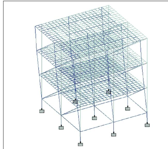
FIG. 4 I MODE IN OUT-OF-PLANE: 4.69 Hz
