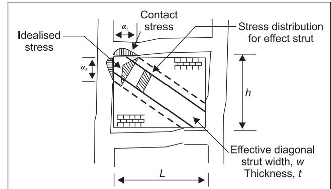
FIG. 2 EQUIVALENT DIAGONAL STRUT (DRYDALE, ET AL. 1994)
