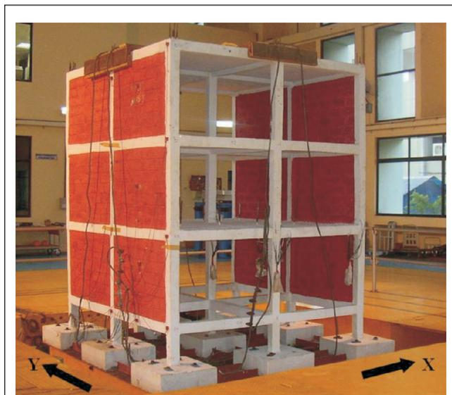
FIG. 7 FIRST 3D MODEL ON SHAKE TABLE
