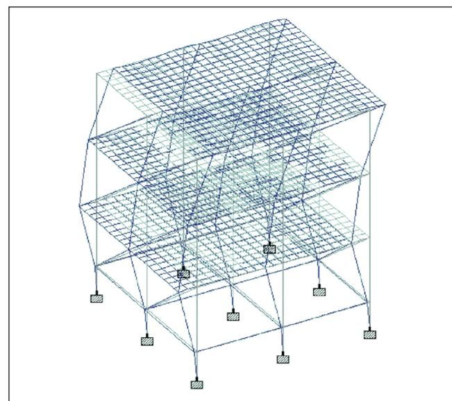
FIG. 6 III MODE IN OUT-OF-PLANE: 15.15 Hz
