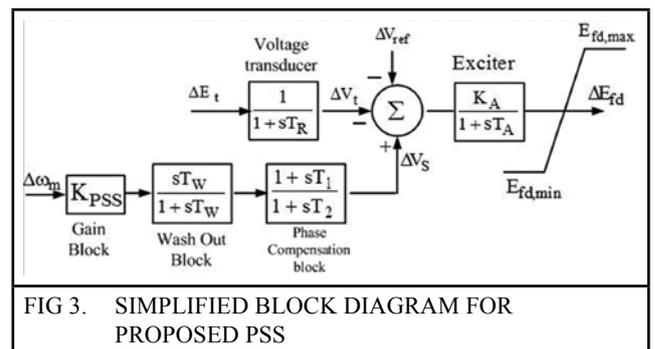
FIG 3. SIMPLIFIED BLOCK DIAGRAM FOR PROPOSED PSS
