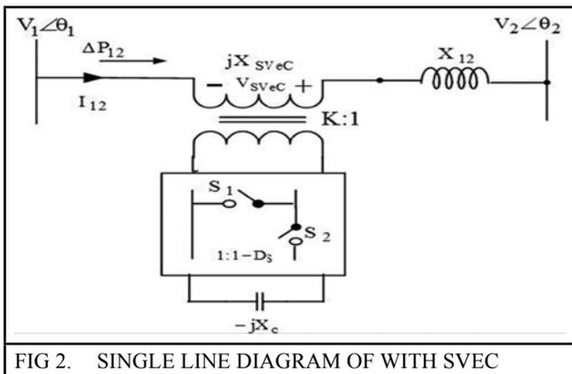
FIG 2. SINGLE LINE DIAGRAM OF WITH SVEC
