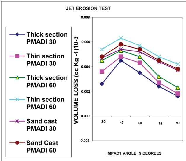
FIG. 1 EROSION VOLUME LOSS OF PMADI SAMPLES.
