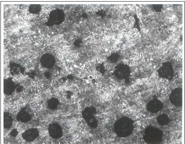
FIG. 6 SAND CAST ADI 60 MIN 200X.
