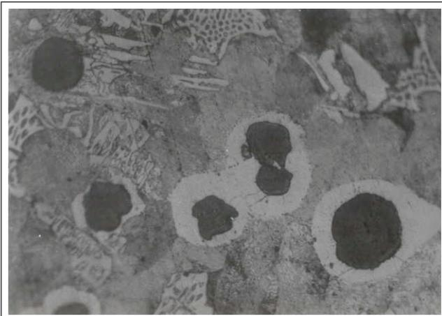
FIG. 3 THICK SECTION PMADI AS CAST 200X.
