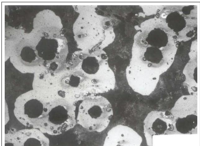
FIG. 2 THIN SECTION AS CAST PMADI SAMPLES 200X.
