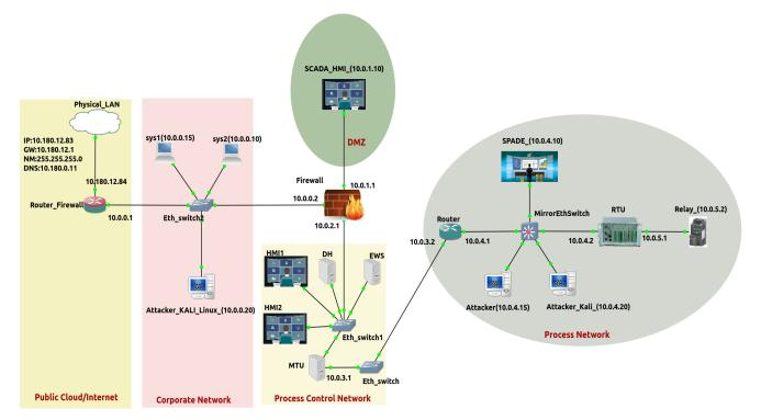
Figure 1. Configurable Hybrid SCADA testbed Architecture.
