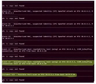
Figure 13. Incident-report for unauthorized port scan.
