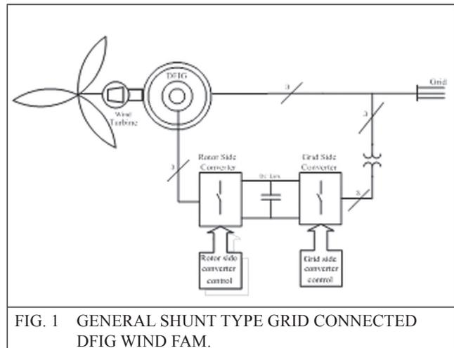
FIG. 1 GENERAL SHUNT TYPE GRID CONNECTED DFIG WIND FARM.
