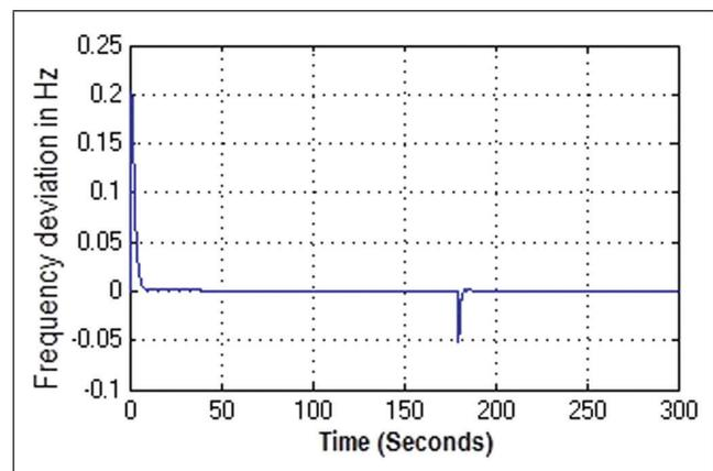
FIG. 5 FREQUENCY RESPONSE OF AREA 1 IN THE PUBLIC SECTOR UNIT WITH PID CONTROLLER.
