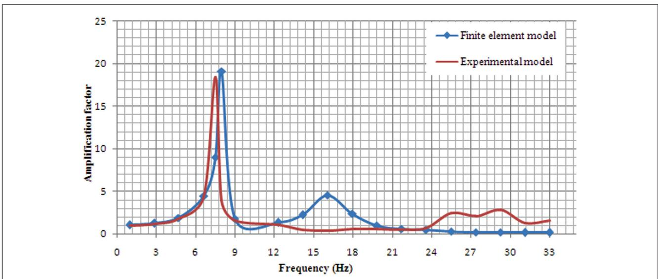
FIG. 3 RESPONSE AMPLIFICATION AT THE TOP OF THE PORCELAIN INSULATOR OF 12 kV CIRCUIT BREAKER IN X-AXIS.
