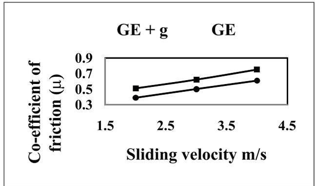
FIG. 4 PLOT OF CO-EFFICIENT OF FRICTION V/S SLIDING VELOCITY FOR G-E AND G-E+G
