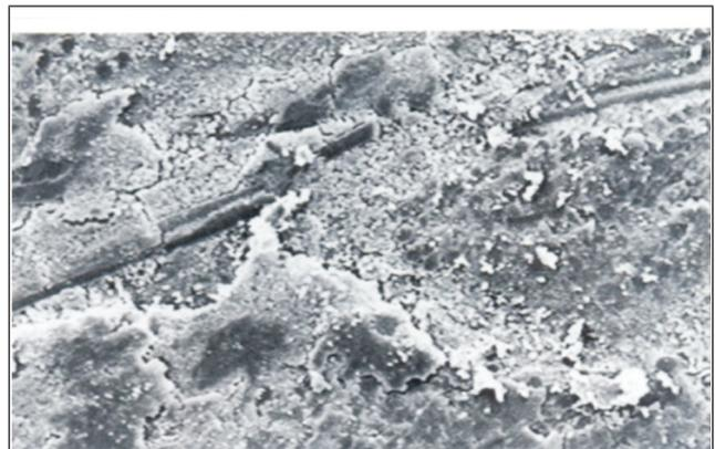
FIG. 6 SLIDE WEAR FEATURES OF G-E SYSTEM FOR 50 N LOAD
