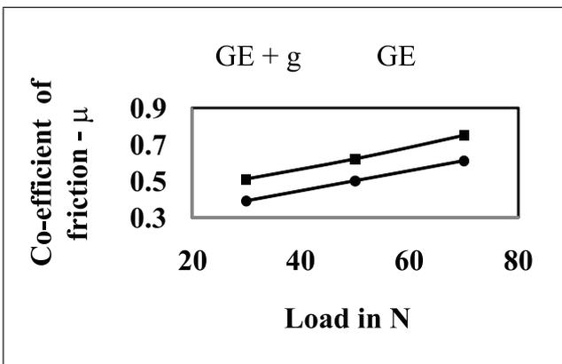
FIG. 3 PLOT OF CO-EFFICIENT OF FRICTION V/S LOAD FOR G-E AND G-E+G
