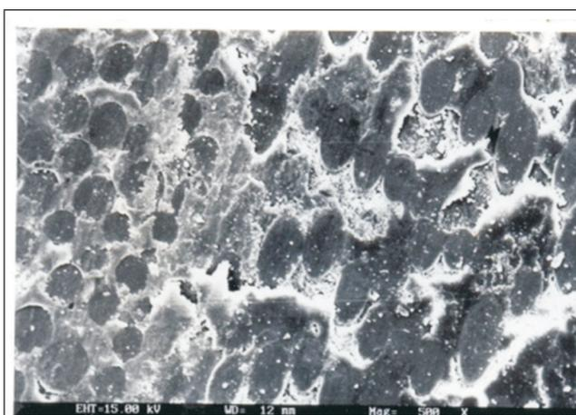
FIG. 9 SLIDE WEAR FEATURES OF G-E + G SYSTEM 50 N LOAD
