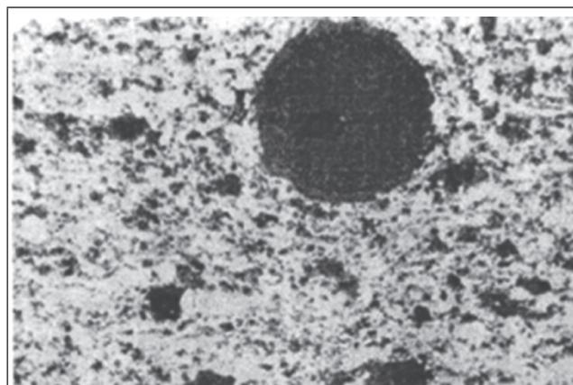
FIG. 3 OPTICAL PHOTOMICROGRAPH OF Fe<sub>3</sub>Al-25VOL.% FLY ASH (X1000)
