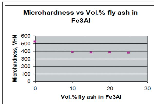
FIG. 2 MICROHARDNESS VS. VOLUME PERCENT OF FLY ASH IN FE<sub>3</sub>AL
