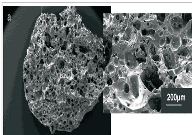
FIG. 4 POROSITY DEVELOPMENT IN FLY ASH BY THERMAL HEATING AT 1150°C [13]
