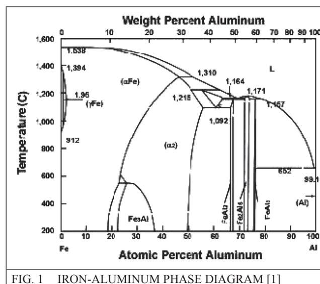
FIG. 1 IRON-ALUMINUM PHASE DIAGRAM [1]
