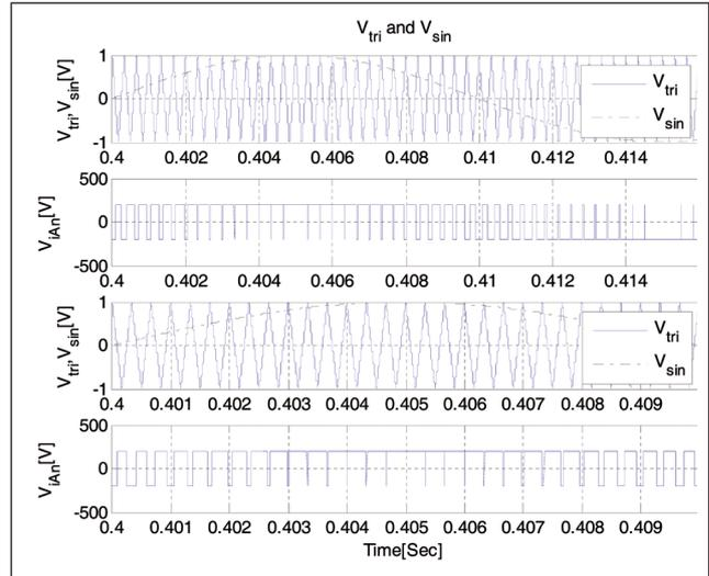
FIG. 6 CARRIER WAVE AND MODULATING WAVE
