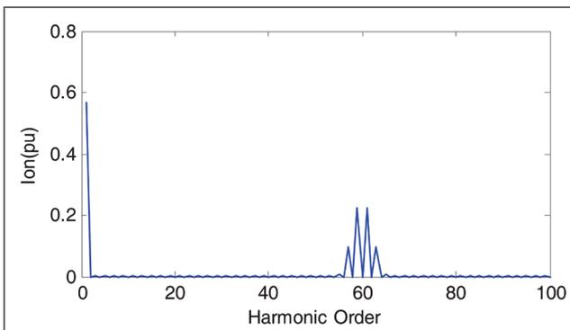
FIG. 17 HARMONIC CONTENT OF OUTPUT CURRENT
