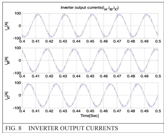
FIG. 8 INVERTER OUTPUT CURRENTS
