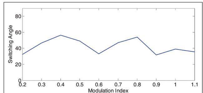
FIG. 14 SWITCHING ANGLE  $\alpha_3$  VS MODULATION INDEX
