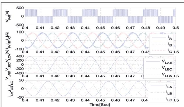
FIG. 11 INVERTER AND LOAD VOLTAGES AND CURRENTS
