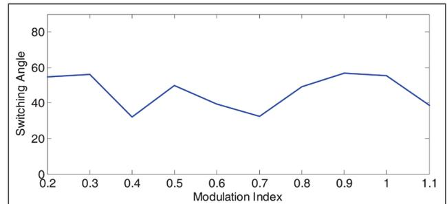
FIG. 12 SWITCHING ANGLE  $\alpha_1$  VS MODULATION INDEX
