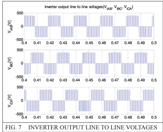
FIG. 7 INVERTER OUTPUT LINE TO LINE VOLTAGES
