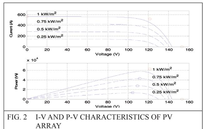
FIG. 2 I-V AND P-V CHARACTERISTICS OF PV ARRAY
