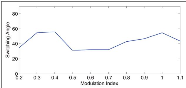
FIG. 15 SWITCHING ANGLE  $\alpha_4$  VS MODULATION INDEX
