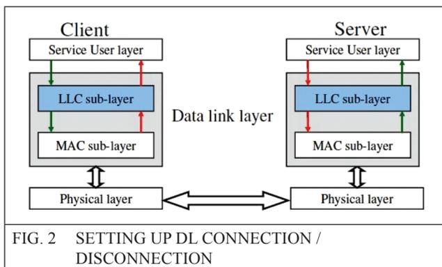
FIG. 2 SETTING UP DL CONNECTION / DISCONNECTION
