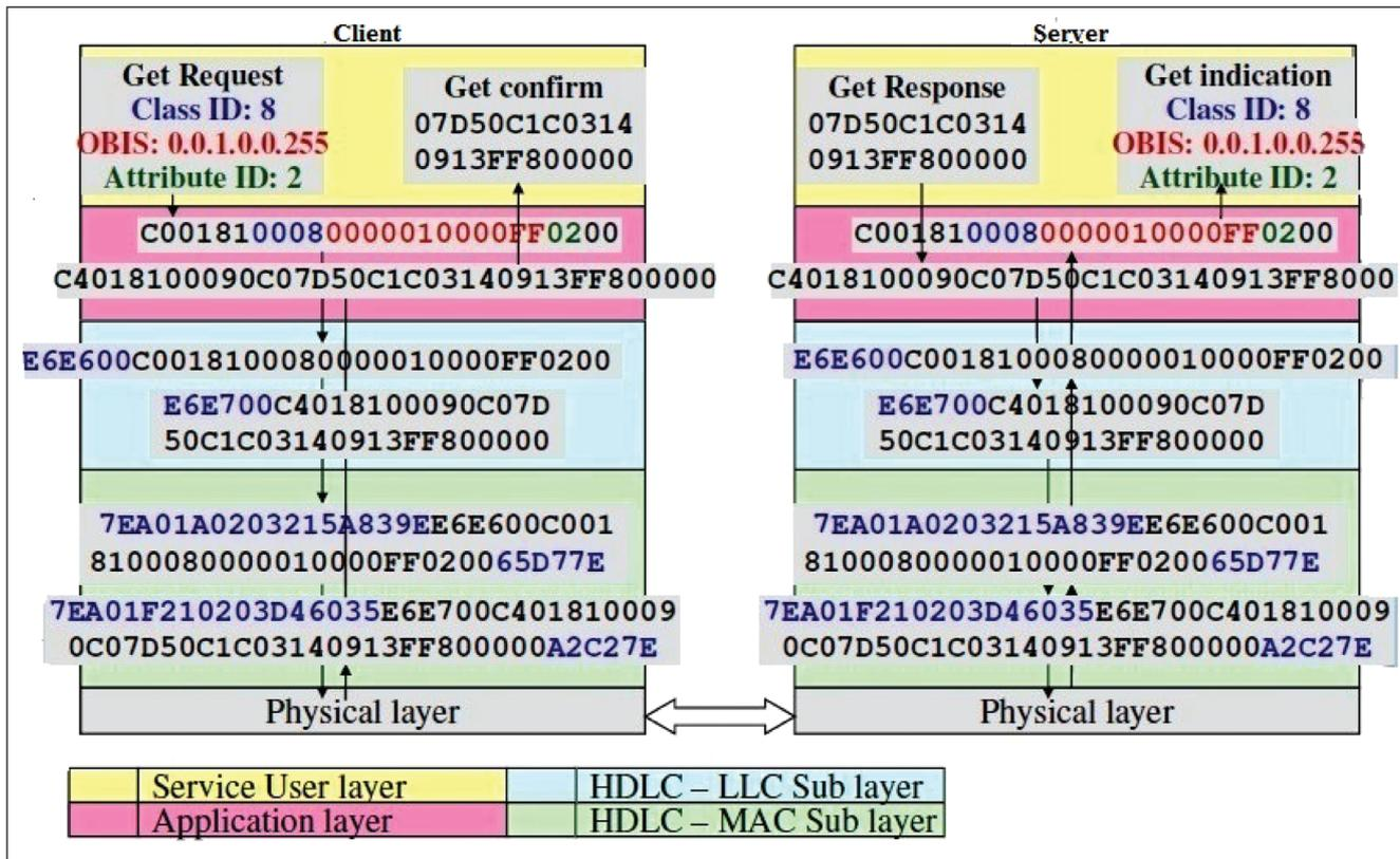
FIG. 4 CONNECTIVITY DIAGRAM BETWEEN SERVER (ENERGY METER) AND CLIENT
