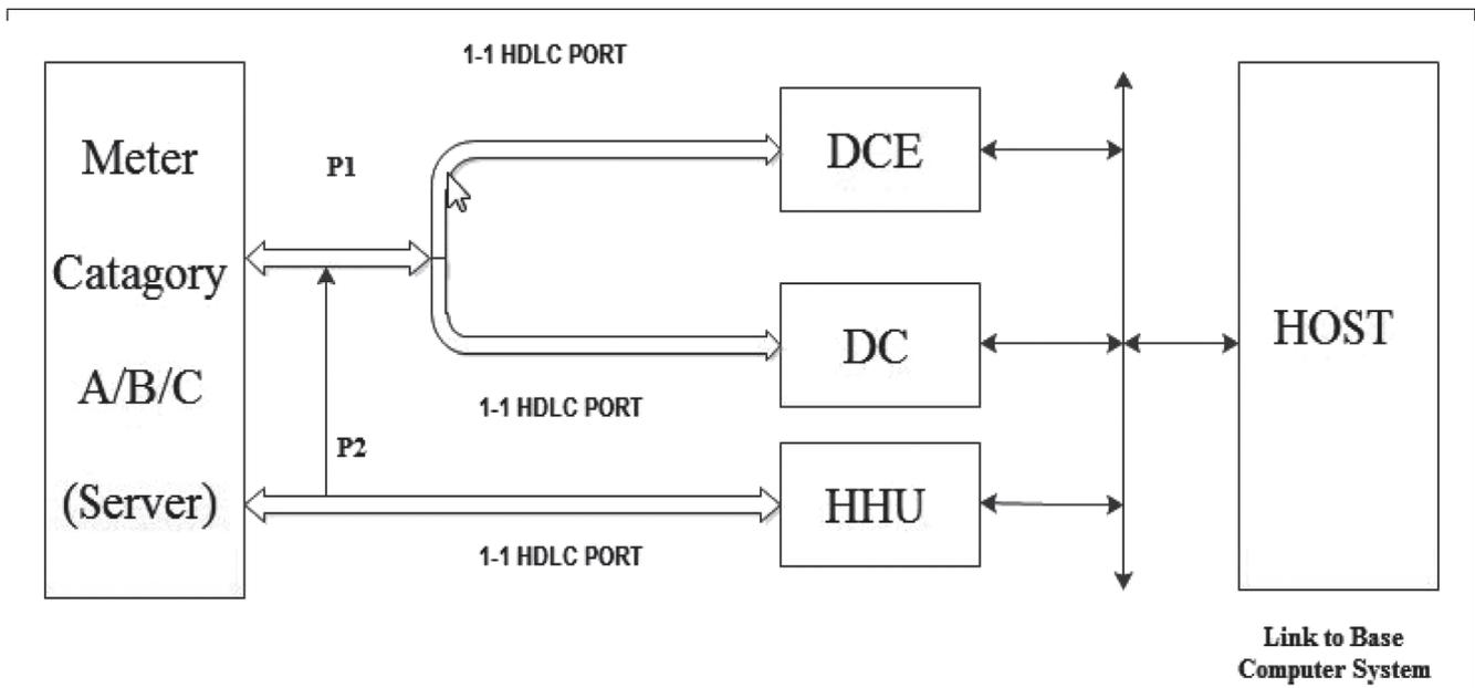
FIG. 1 CONNECTIVITY DIAGRAM BETWEEN SERVER (ENERGY METER) AND CLIENT
