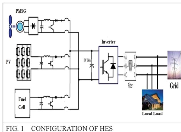
The configuration of hybrid energy system is shown in Figure 1, it contains wind, photovoltaic and fuel cell power system connected to the grid. But in general case hybrid energy system can be a combination of different renewable/non renewable energy systems.
