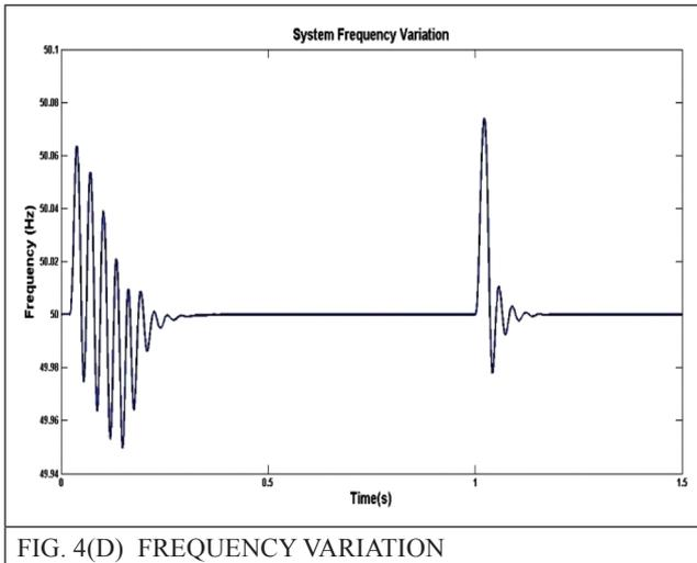
In Figure 4(b), PV & wind current & the system voltages are constant; the change in load current due to load variation is shared by the grid as shown. In Figure 4(c), load active & reactive powers change at 1s from 100 KW to 150 KW & 60 kVAR to 90 kVAR that increased demand is shared by grid as shown. The Figure 4(d) shows the system frequency variation throughout the simulation time & it is within the limit of grid connection requirement, which is specified in the standard IEEE-1547 [4].
