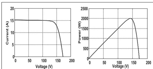
FIG. 2 CHARACTERISTIC OF PV ARRAY UNDER RATED CONDITION OF TEMPERATURE AND SOLAR INSOLATION
