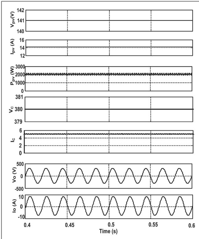
FIG. 5 PERFORMANCE OF THE SYSTEM WITH LINEAR LOAD CHANGES AT T=0.3S
