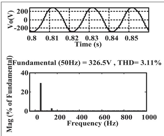
FIG. 6 HARMONIC ANALYSIS OF THE OUTPUT VOLTAGE IN LINEAR LOAD CONDITIONS
