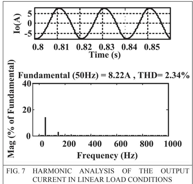
FIG. 7 HARMONIC ANALYSIS OF THE OUTPUT CURRENT IN LINEAR LOAD CONDITIONS
