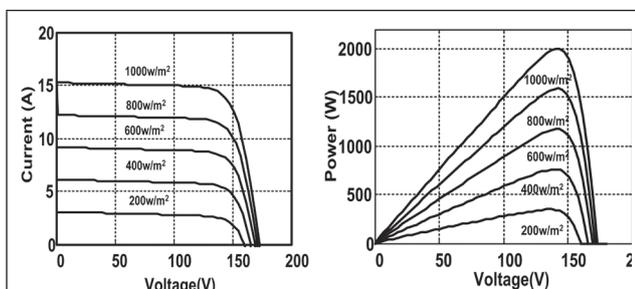
FIG. 3 CHARACTERISTIC OF PV MODULE UNDER CHANGING CONDITIONS OF SOLAR INSOLATION
