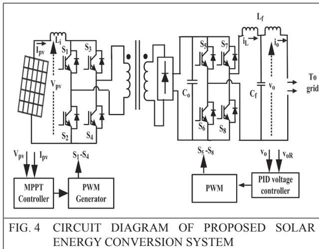
FIG. 4 CIRCUIT DIAGRAM OF PROPOSED SOLAR ENERGY CONVERSION SYSTEM
