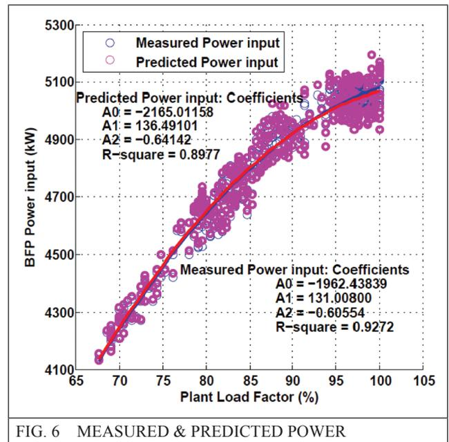
FIG. 6 MEASURED & PREDICTED POWER
