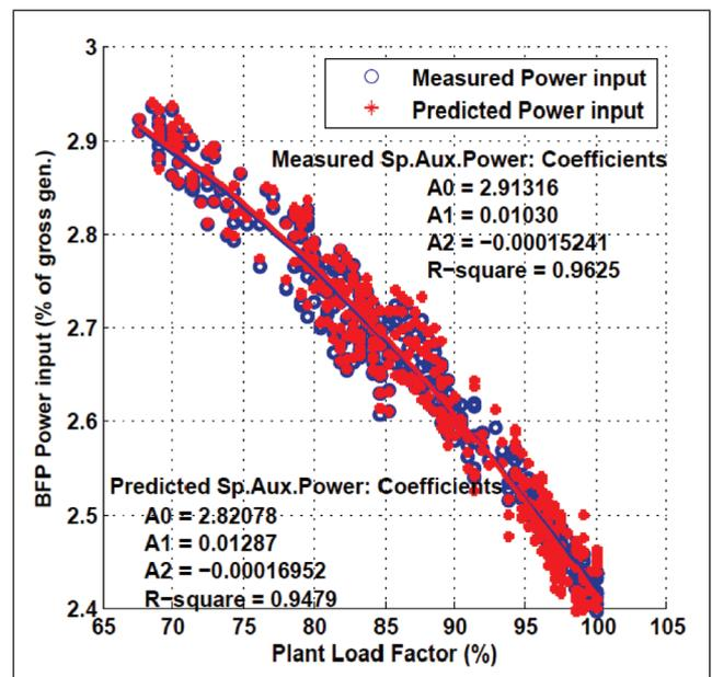
FIG. 7 MEASURED & PREDICTED SPECIFIC AUXILIARY POWER
