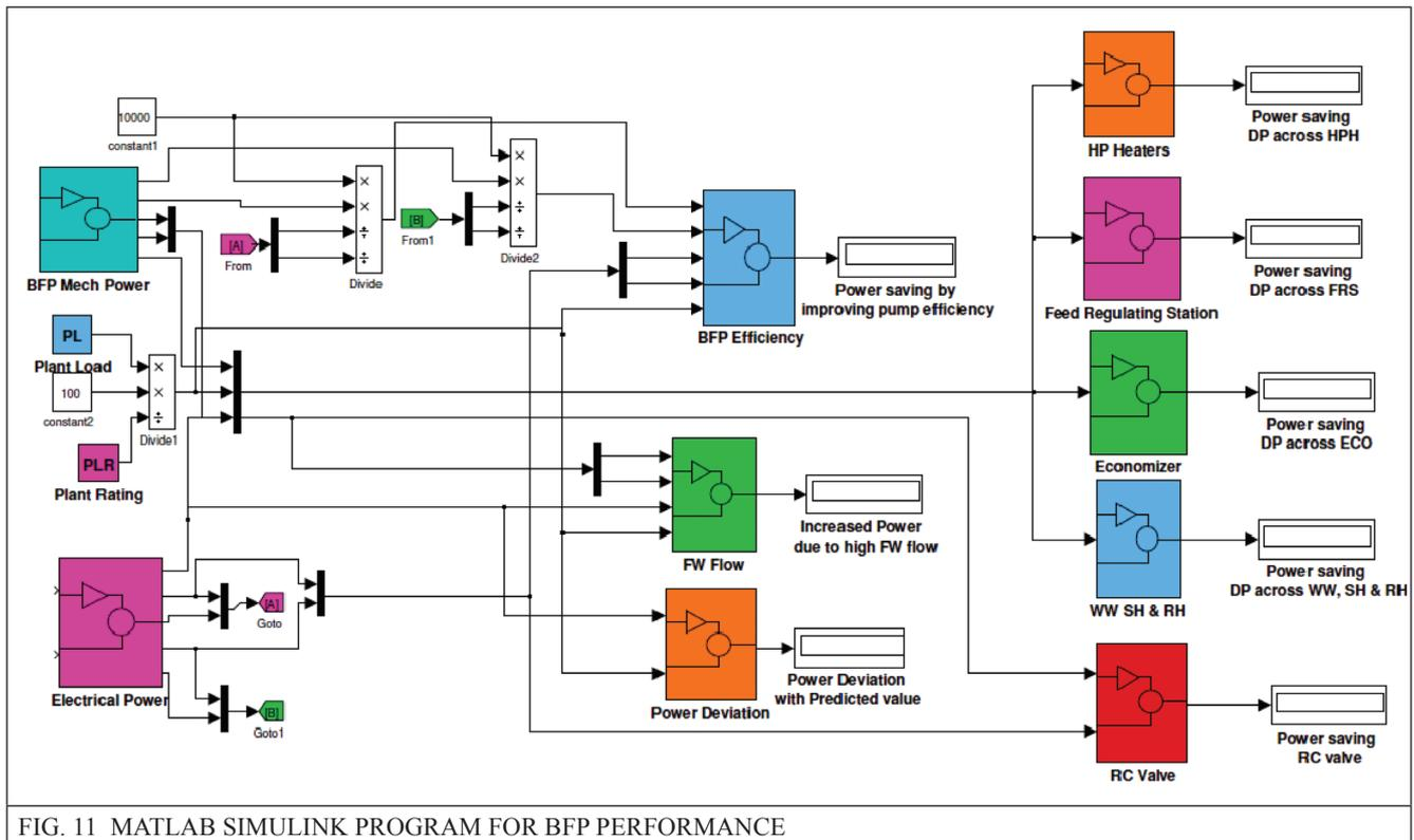
FIG. 11 MATLAB SIMULINK PROGRAM FOR BFP PERFORMANCE
