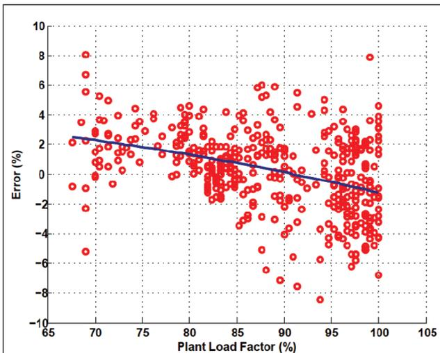
FIG. 8 ERROR BETWEEN MEASURED & PREDICTED POWER
