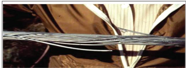
FIG. 1 VIEW OF BROKEN STRANDS OF CONDUCTORS
