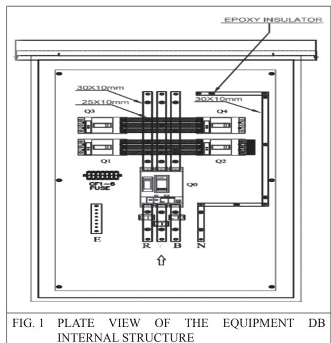
FIG. 1 PLATE VIEW OF THE EQUIPMENT DB INTERNAL STRUCTURE
