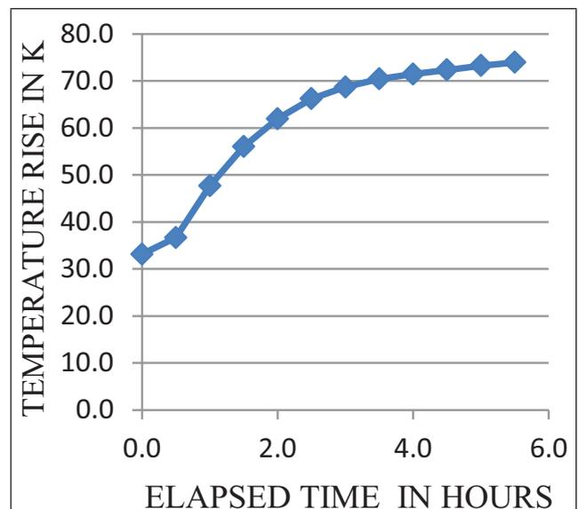
FIG. 7 THERMAL PROFILE OF SUPPORT INSULATOR
