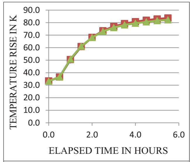
FIG. 6 THERMAL PROFILE OF BUSBAR JOINTS
