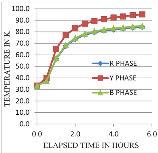
FIG. 4 THERMAL PROFILE OF PANEL INCOMING TERMINAL
