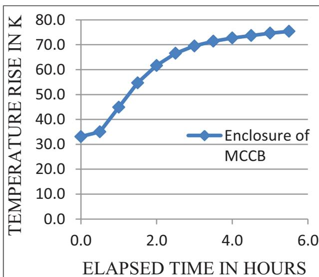
FIG. 8 THERMAL PROFILE OF MCCB ENCLOSURE
