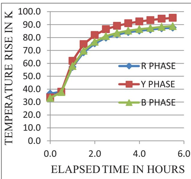
FIG. 5 THERMAL PROFILE OF MAIN BREAKER INCOMING
