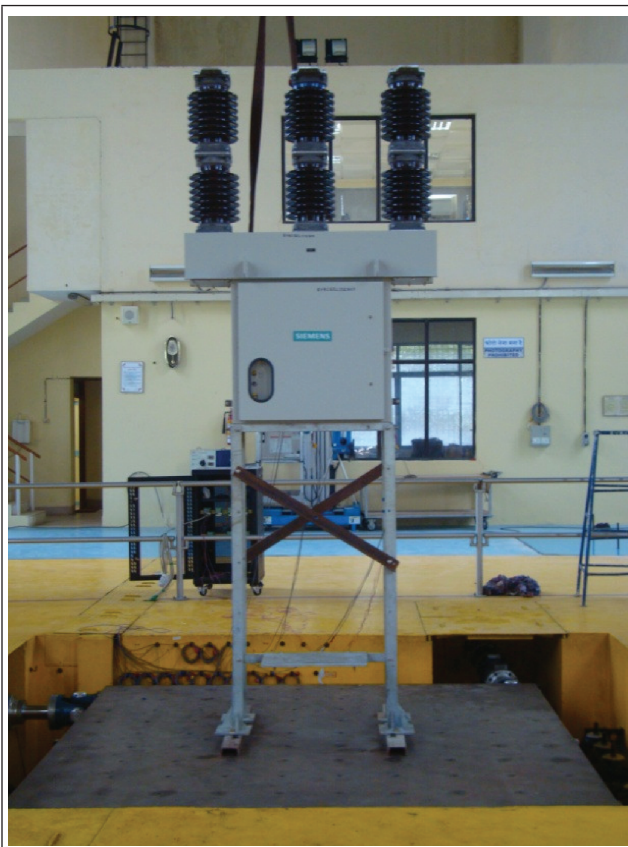
FIG. 1 CIRCUIT BREAKER WITH SUPPORT STRUCTURE MOUNTED ON SHAKE TABLE
