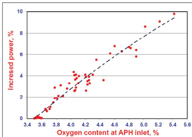
FIG. 11 INCREASED POWER PA FANS WITH HIGHER EXCESS AIR
