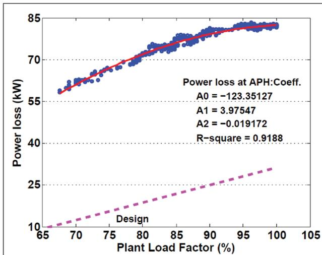
FIG. 5 VARIATION OF POWER LOSS IN APH WITH PLF
