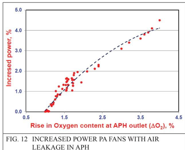
FIG. 12 INCREASED POWER PA FANS WITH AIR LEAKAGE IN APH
