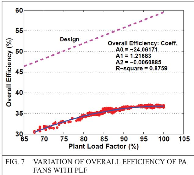
FIG. 7 VARIATION OF OVERALL EFFICIENCY OF PA FANS WITH PLF
