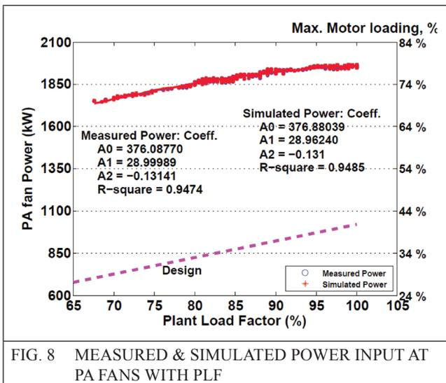
FIG. 8 MEASURED & SIMULATED POWER INPUT AT PA FANS WITH PLF
