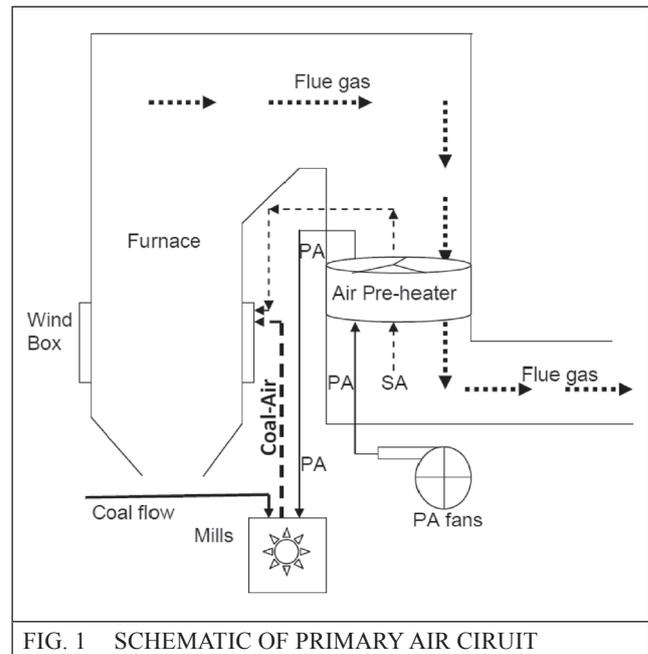
FIG. 1 SCHEMATIC OF PRIMARY AIR CIRCUIT
