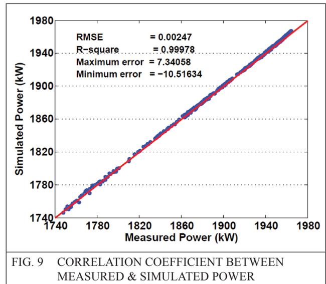
FIG. 9 CORRELATION COEFFICIENT BETWEEN MEASURED & SIMULATED POWER
