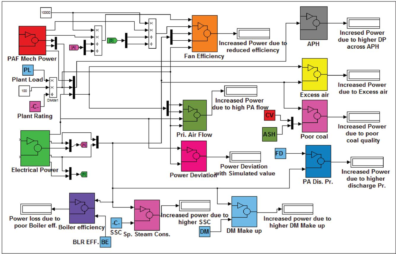
FIG. 10 MATLAB SIMULINK PROGRAM FOR PA FANS
