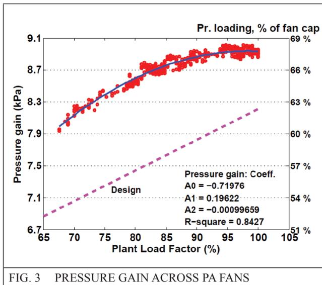
FIG. 3 PRESSURE GAIN ACROSS PA FANS
