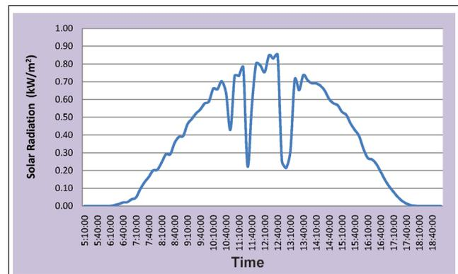
FIG. 6 VARIATIONS IN SOLAR RADIATION RESULTING IN RAMPING OF THE STEAM TURBINE
