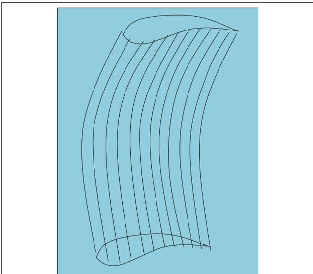
FIG. 4 VIEW OF A 3-D TAPERED BLADE WITH BOWING
