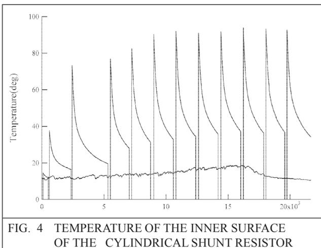
FIG. 4 TEMPERATURE OF THE INNER SURFACE OF THE CYLINDRICAL SHUNT RESISTOR
