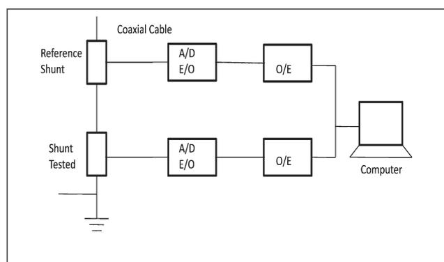
FIG. 8 ARRANGEMENT OF THE SHUNT TESTED
