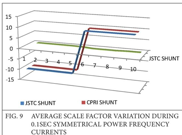
**4.2.2 Linearity tests with power frequency current**
