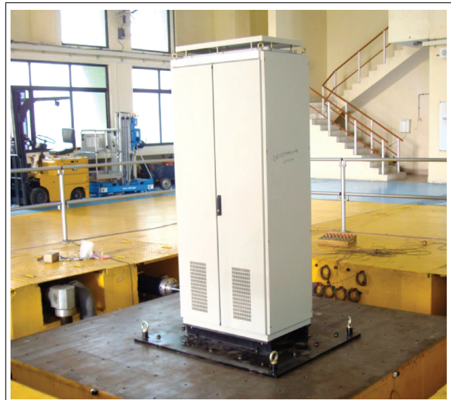
FIG. 1 ELECTRICAL CABINET MOUNTED ON TRI-AXIAL SHAKE TABLE
