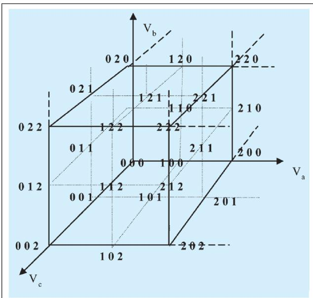
FIG. 2 3D SPACE VECTORS OF A THREE LEVEL INVERTER
