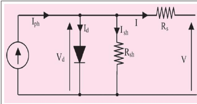
FIG. 7 PV CELL MODELLING
