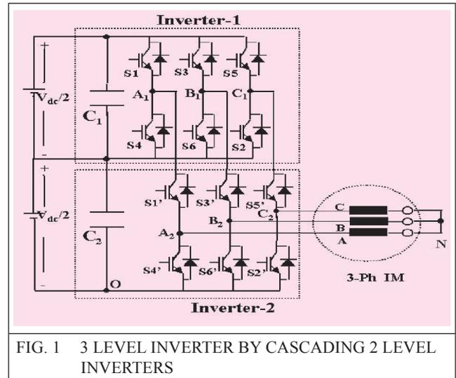
FIG. 1 3 LEVEL INVERTER BY CASCADING 2 LEVEL INVERTERS
