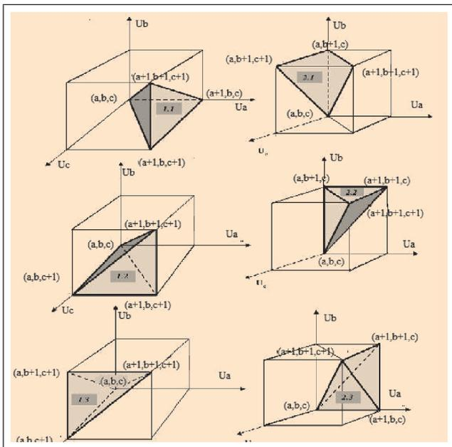
FIG. 4 TETRAHEDRONS IN TO THE CUBE WITH THE CORRESPONDING STATE VECTORS
