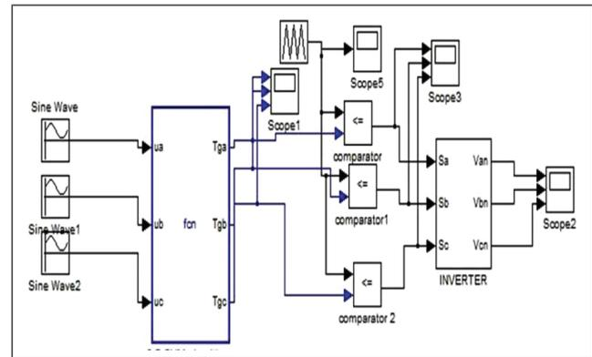
FIG. 5 SIMULATION DIAGRAM OF TWO LEVEL INVERTER WITH 3D SVM
