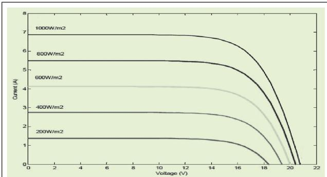
FIG. 8 VARIATION OF VOLTAGE AND CURRENT OF SOLAR PV OUTPUT WITH VARIATION IN INSOLATION
