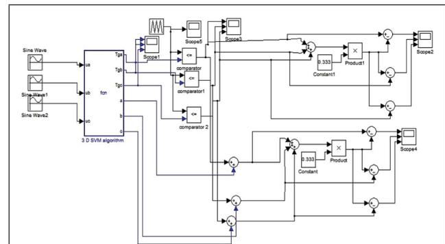
FIG. 6 SIMULATION DIAGRAM OF THREE LEVEL INVERTER WITH 3D SVM
