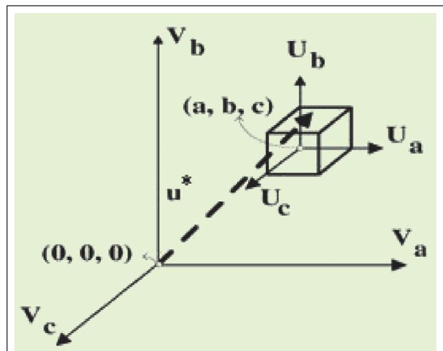
FIG. 3 ORIGIN OF THE SUB CUBE WHERE THE REFERENCE VECTOR IS SUPPOSED TO BE FOUND.
