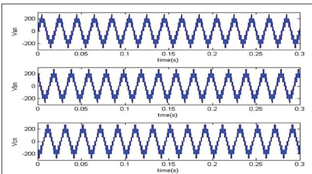
FIG. 9 OUTPUT AC WAVEFORM OF MULTI LEVEL INVERTER USING THE PROPOSED TECHNIQUE
