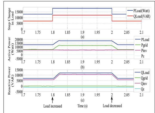
FIG. 9 EFFECT OF VARIATION IN LOAD DEMAND DURING SHADING PATTERN SP2: (A) STEP CHANGE IN LOAD (B) ACTIVE POWER OF THE LOAD, INVERTER, GRID AND RIPPLE FILTER (C) REACTIVE POWER OF THE LOAD, PV INVERTER, GRID AND RIPPLE FILTER
