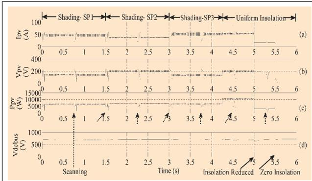
FIG. 6 PV SIDE WAVEFORMS DURING GPP TRACKING: (A) OUTPUT CURRENT (IPV) (B) OUTPUT VOLTAGE (VPV) (C) OUTPUT POWER (PPV) AND (D) DC LINK VOLTAGE
