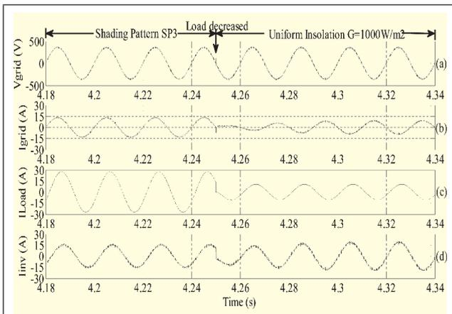
FIG. 11 EFFECT OF SIMULTANEOUS CHANGE IN SHADING AND LOAD ON PARAMETERS OF PHASE-A: (A) GRID VOLTAGE (B) GRID CURRENT (C) LOAD CURRENT AND (D) PV INVERTER CURRENT
