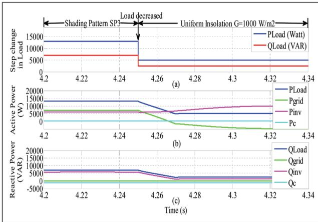
FIG. 10 EFFECT OF SIMULTANEOUS VARIATION IN INSOLATION AND LOAD: (A) ACTIVE POWER OF THE LOAD, GRID, INVERTER AND RIPPLE FILTER (B) REACTIVE POWER OF THE LOAD, GRID, INVERTER AND RIPPLE FILTER
