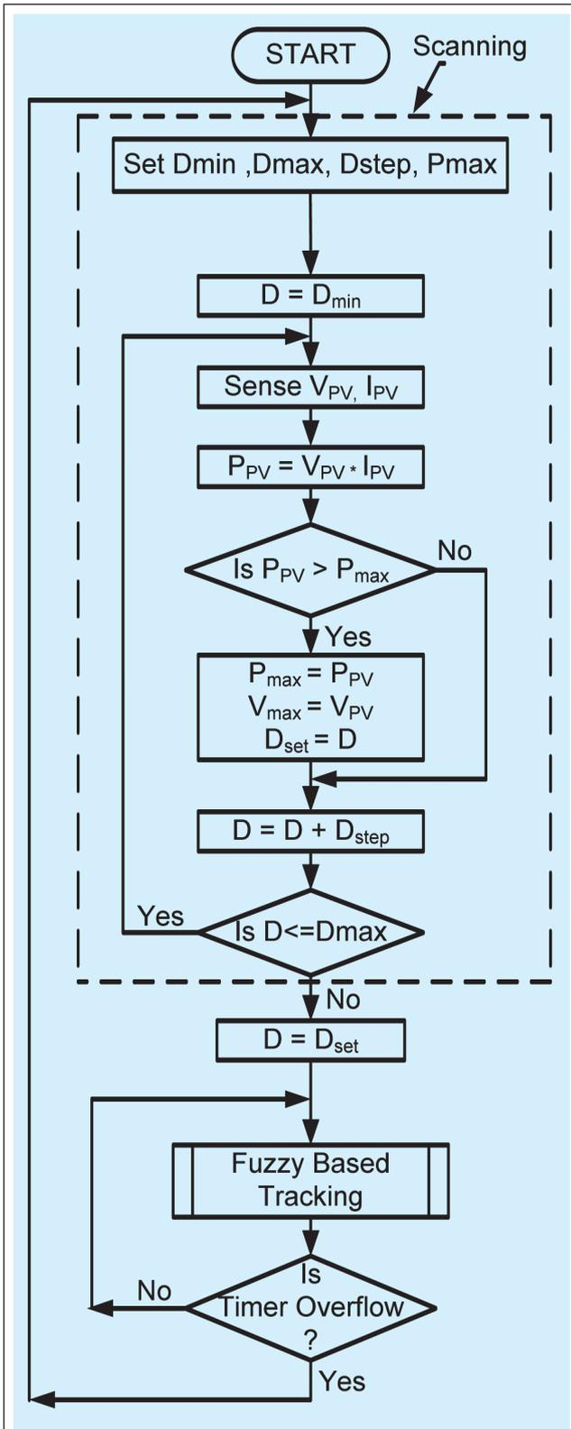
FIG. 2 FLOWCHART OF PROPOSED GPP TRACKING TECHNIQUE
