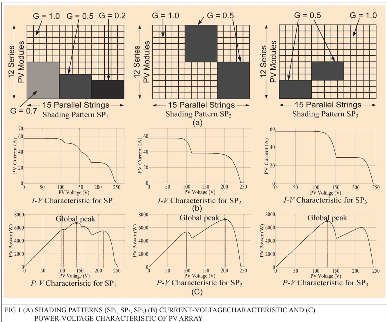
FIG.1 (A) SHADING PATTERNS (SP<sub>1</sub>, SP<sub>2</sub>, SP<sub>3</sub>) (B) CURRENT-VOLTAGE CHARACTERISTIC AND (C) POWER-VOLTAGE CHARACTERISTIC OF PV ARRAY
