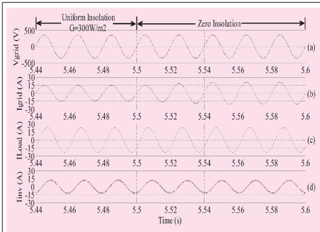
FIG. 8 EFFECT OF VARIATION IN INSOLATION FROM UNIFORM TO ZERO ON PARAMETERS OF PHASE-A: (A) GRID VOLTAGE (B) GRID CURRENT (C) LOAD CURRENT AND (D) INVERTER CURRENT
