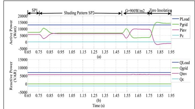
FIG. 7 EFFECT OF VARIATION IN PARTIAL SHADOWING CONDITION WITH CONSTANT LOAD: (A) ACTIVE POWER OF LOAD, INVERTER, GRID AND RIPPLE FILTER (W) (B) REACTIVE POWER OF LOAD, INVERTER, GRID AND RIPPLE FILTER (VAR)
