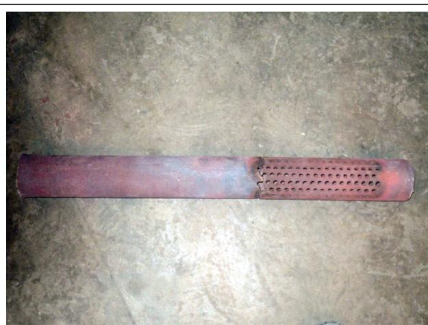
FIG. 4 IMAGE OF BROKEN INJECTOR TAKEN OUT FROM ATTEMPERATOR
