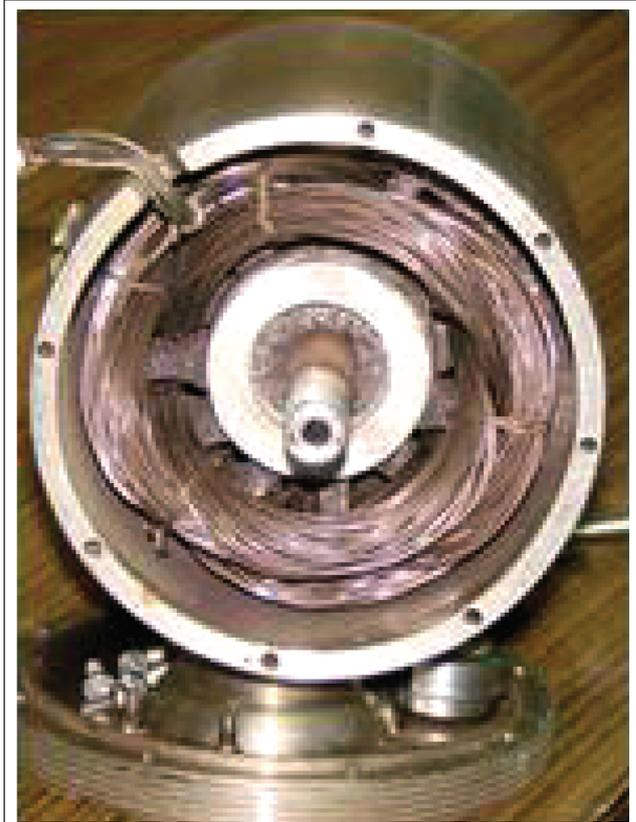
FIG. 12 STATOR OF LOW POWER MOTOR WITH MI CABLE
