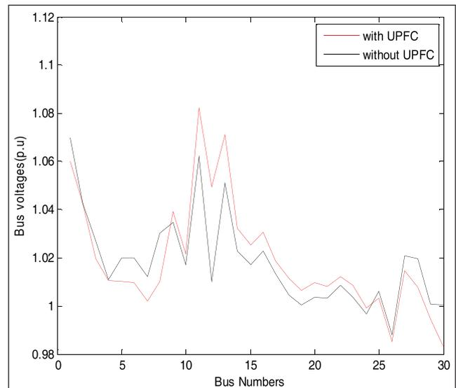
FIG. 4 VOLTAGE PROFILE OF IEEE 30 BUS SYSTEM
