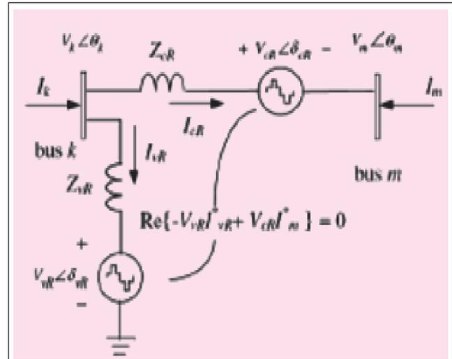
FIG. 1 UPFC EQUIVALENT CIRCUIT
