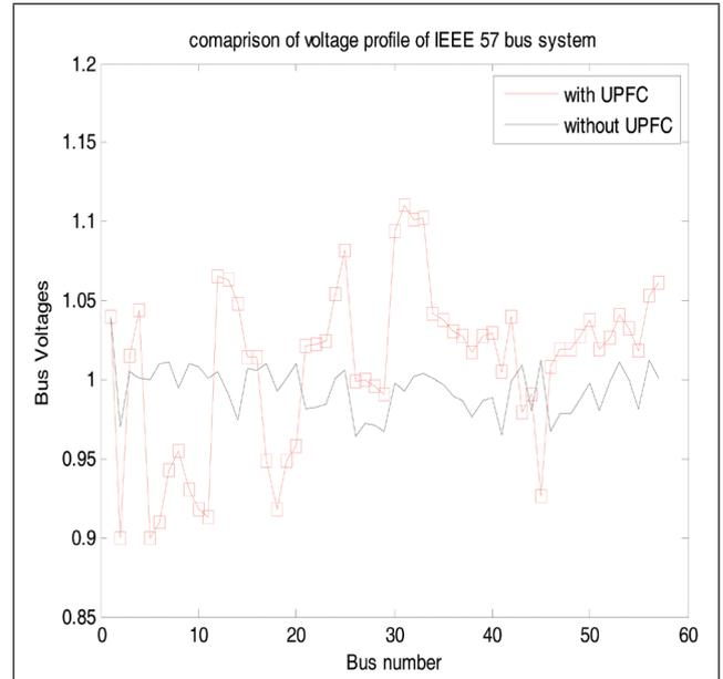
FIG. 7 VOLTAGE PROFILE OF IEEE 57 BUS WITH AND WITHOUT UPFC
