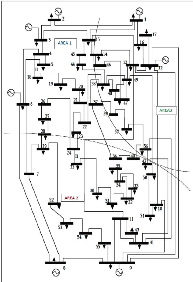
FIG. 5 SINGLE LINE DIAGRAM OF IEEE 57 BUS SYSTEM
