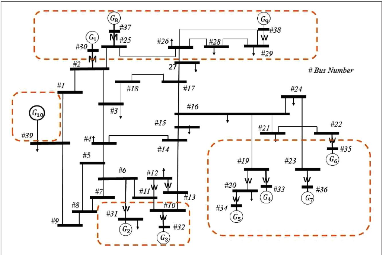
FIG. 5 SINGLE LINE DIAGRAM OF 10 GENERATORS AND 39 BUS POWER SYSTEM (IEEE 39 BUS SYSTEM)
