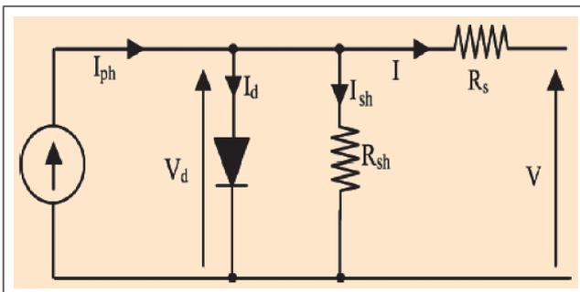
FIG. 5 MODELING OF SOLAR PV.
