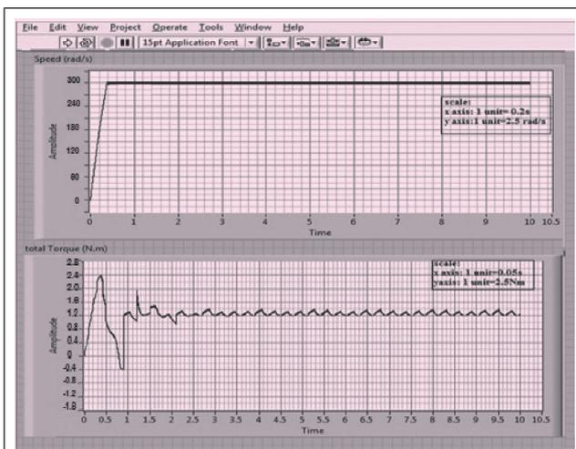
FIG. 12 SPEED SETPOINT AT 3000 RPM FOR RATED TORQUE OUTPUT
