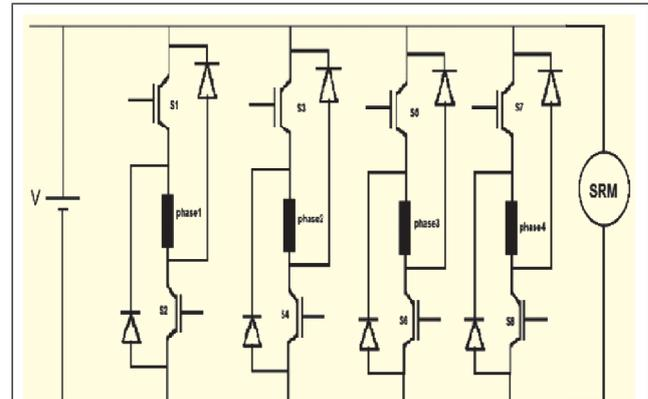
FIG. 3 CONVERTER CONFIGURATION.
