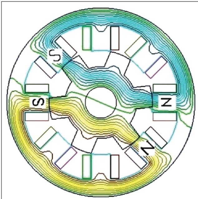
FIG. 2 CONSTRUCTION AND FIELD ORIENTATION OF SRM.
