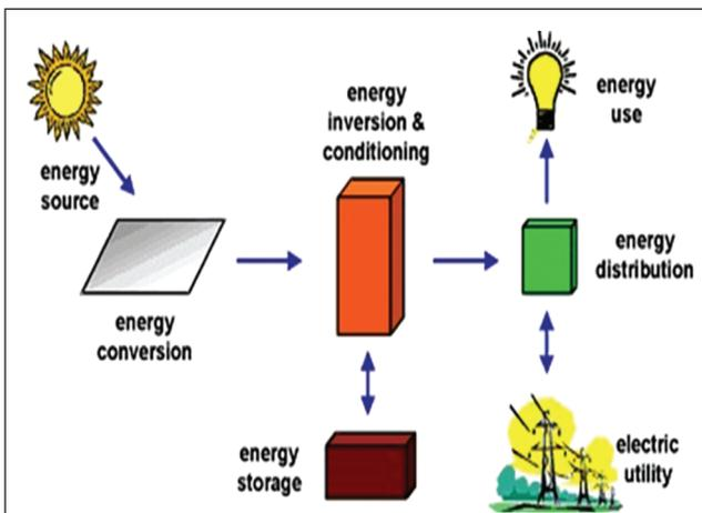
FIG. 1 GENERAL SCHEMATIC OF A SOLAR PV BASED POWER GENERATION SYSTEM.
