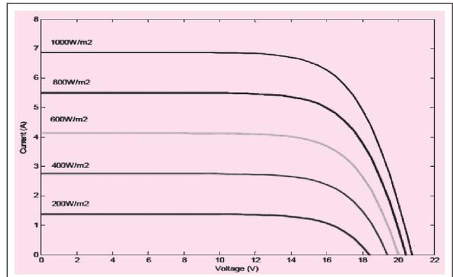
FIG. 7 PV CELL SIMULATION OUTPUT
