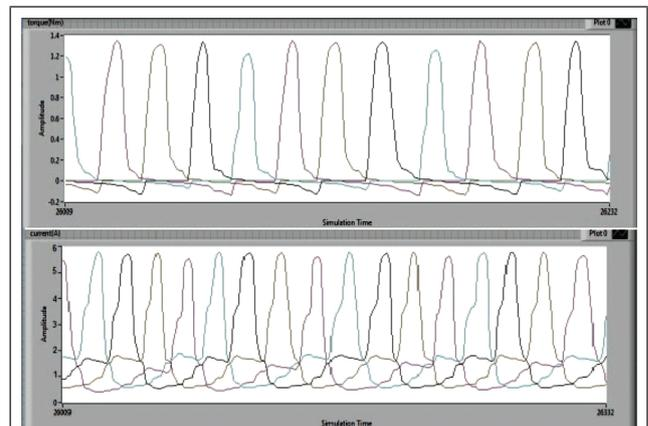
FIG. 11 DEVELOPED TORQUE AND CURRENT WAVEFORMS FOR FOUR PHASES OF SRM
