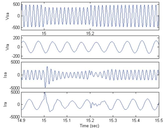
**Figure 2.** Voltage and current of stator and rotor at the fault duration of 15 to 15.2 sec<sup>7</sup>.
