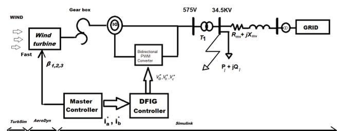
Figure 1. Structure of the variable-speed wind turbine with DFIG and grid connection.
