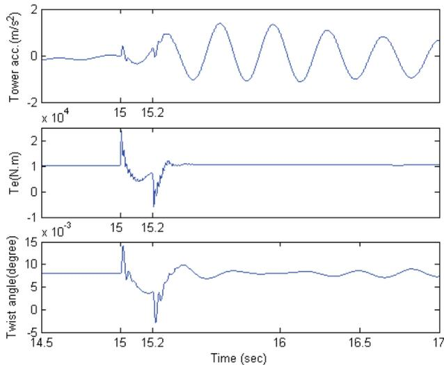
**Figure 4.** The effect of voltage SAG on generator torque during fault duration 15 to 15.2 sec<sup>2</sup>.
