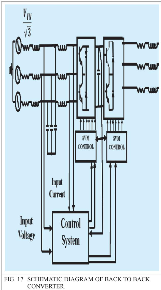
The switching frequencies of the two converters are related to the adopted modulation strategies and should be chosen with care in order to make a fair comparison. Furthermore, both converters need an input filter to reduce the input current harmonics, and the filter parameters are strictly related to the switching frequency converter.
