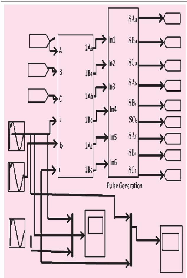
FIG. 21 PULSE GENERATION TO CONTROL MATRIX CONVERTER SWITCHES
