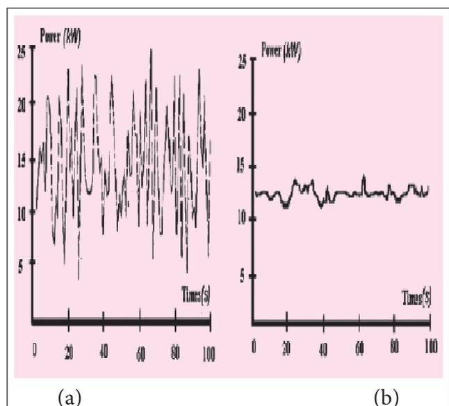
FIG. 2 POWER OUTPUT DISTURBANCE OF A TYPICAL WIND TURBINE WITH (A) CONSTANT-SPEED, (B) VARIABLE-SPEED
