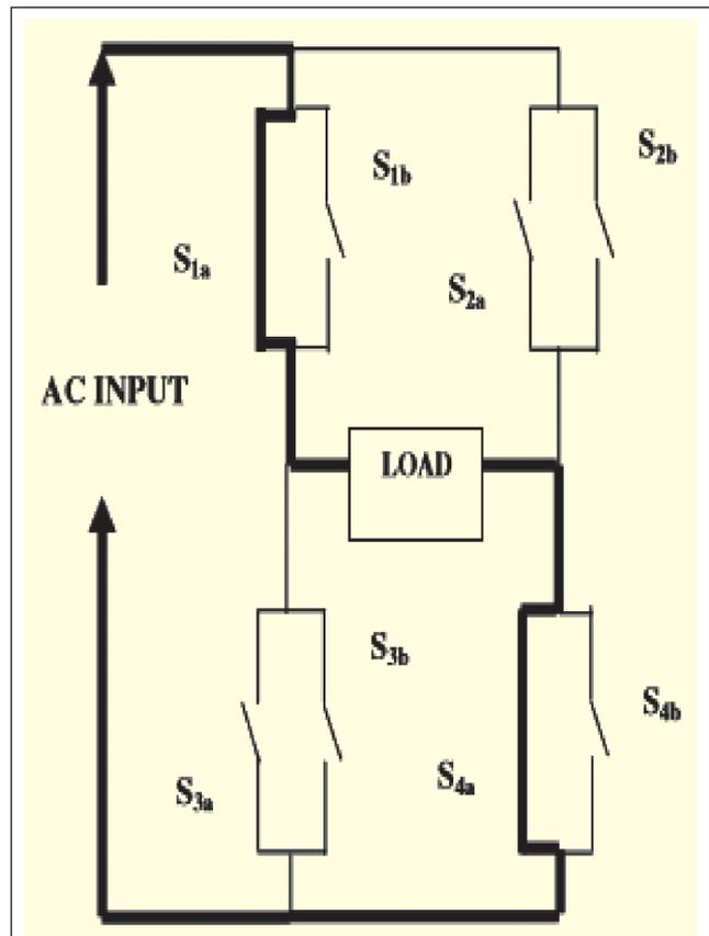
FIG. 5  $S_{1A}$  AND  $S_{3A}$  SWITCHED ON DURING POSITIVE HALF CYCLE
