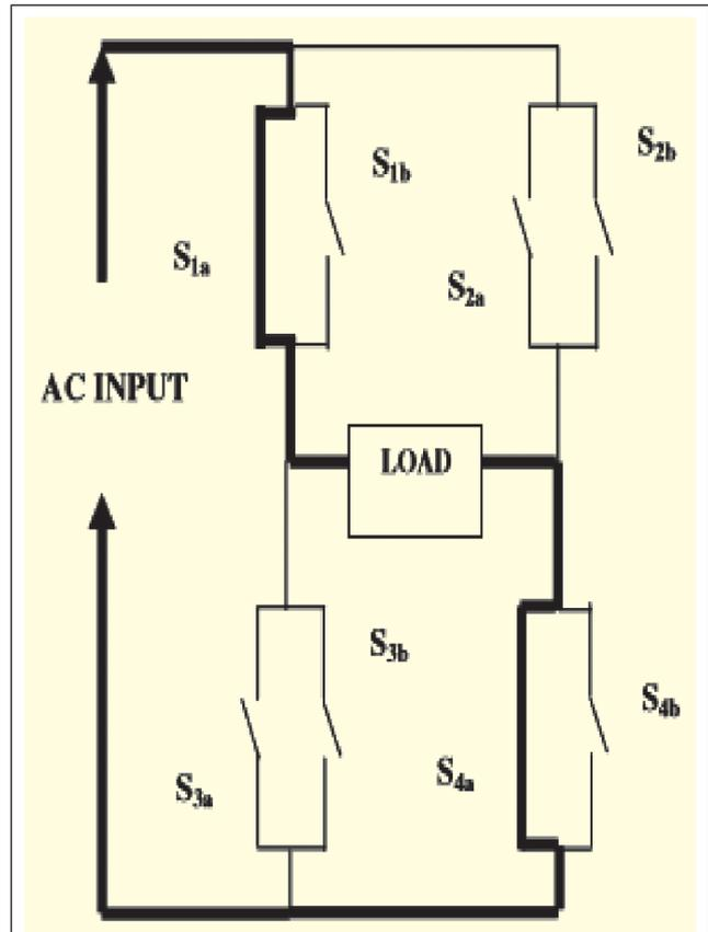
FIG. 5  $S_{1A}$  AND  $S_{4A}$  SWITCHED ON DURING POSITIVE HALF CYCLE
