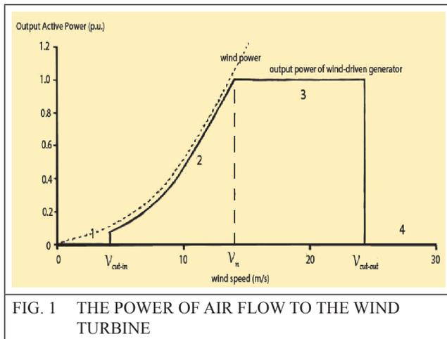
FIG. 1 THE POWER OF AIR FLOW TO THE WIND TURBINE
