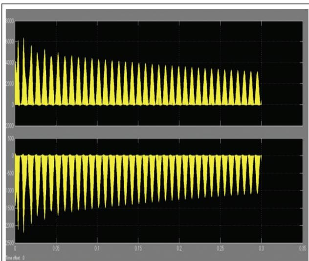
FIG. 30 ACTIVE AND REACTIVE POWER AT THE SENDING END
