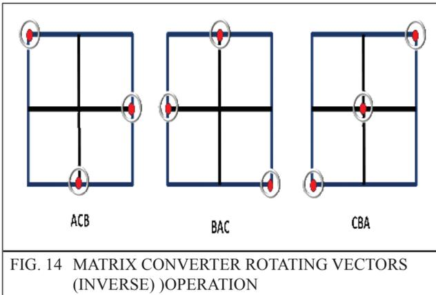
Figure 14 shows inverse operating state vectors of three phase matrix converter. In this way one phase is rotated in such a way that it connects all the output phase in a cycle of operation. This operation may be selected during reverse operation of induction motor
