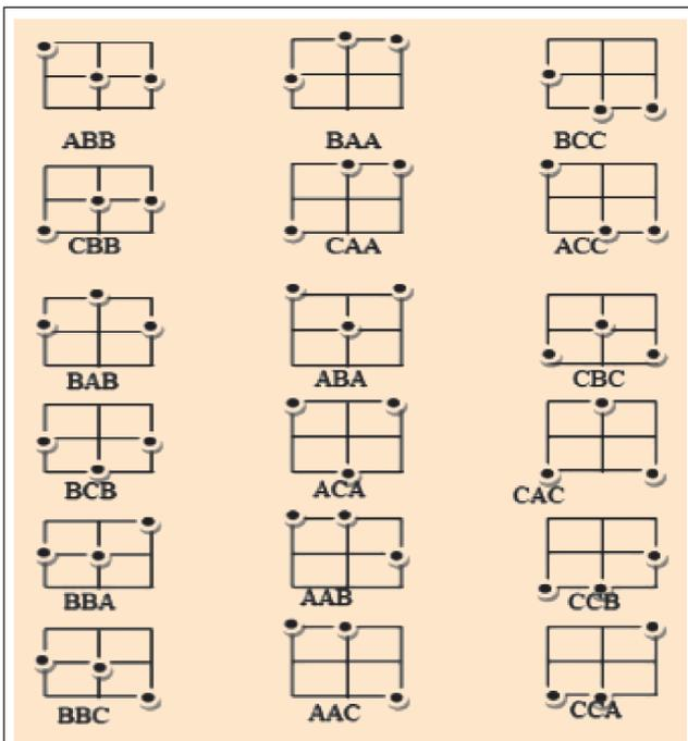
FIG. 15 MATRIX CONVERTER ACTIVE VECTORS (PULSATING)
