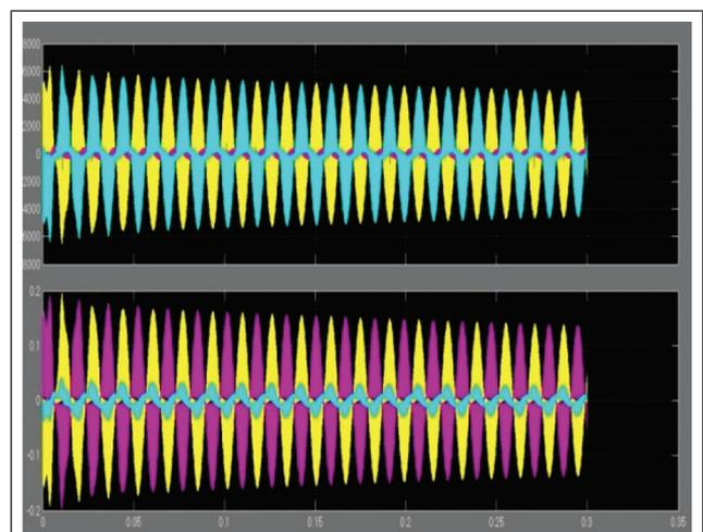
FIG. 28 THREE PHASE WAVEFORM AT THE SENDING END
