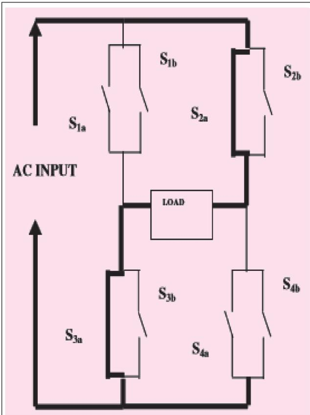
FIG. 7 S<sub>2A</sub> AND S<sub>3A</sub> SWITCHED ON DURING POSITIVE HALF CYCLE
