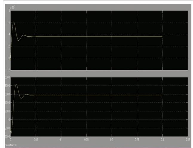
FIG. 31 ACTIVE AND REACTIVE POWER AT THE RECEIVING END
