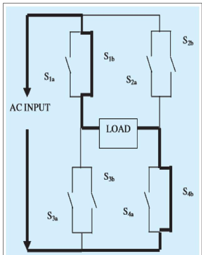
FIG. 6  $S_{1B}$  AND  $S_{3B}$  SWITCHED ON DURING NEGATIVE HALF CYCLE
