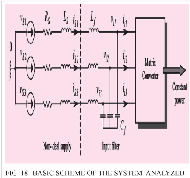
FIG. 18 BASIC SCHEME OF THE SYSTEM ANALYZED
