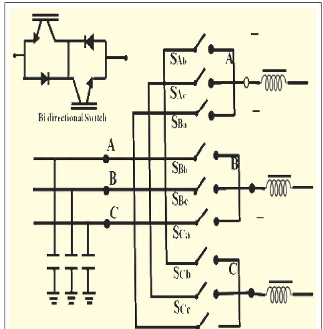
FIG. 10 CIRCUIT SCHEME OF A THREE PHASE MATRIX CIRCUIT CONVERTER
