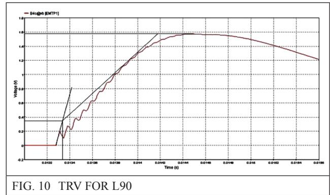
The TRV characteristic for short line fault (L90) for the typical Indian system is shown in Figure 10 above. The TRV peak ( $U_c$ ) in this case was found to be 1592.1 kV peak and the RRRV was 3.99 kV/ $\mu$ s. For the case of transformer limited fault, the TRV peak and RRRV was found to be 1664.5 kV peak and 12.46 kV/ $\mu$ s respectively (Figure 11). These values are well within those specified by standards [2-3] i.e. 1799 kV peak for TRV and 16.1 to 18.0 kV/ $\mu$ s for RRRV.
