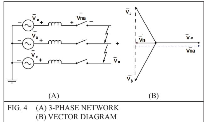
FIG. 4 (A) 3-PHASE NETWORK (B) VECTOR DIAGRAM
