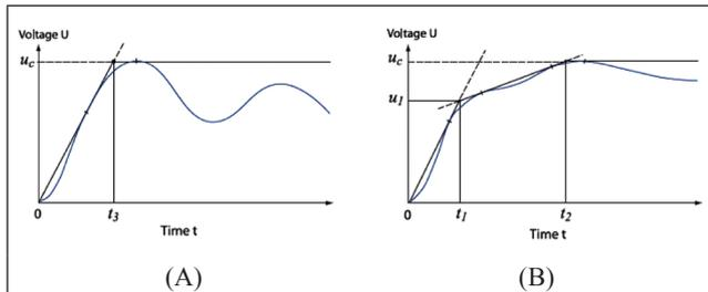
FIG. 3 TRV (A) 2 PARAMETER (B) 4 PARAMETER METHODS
