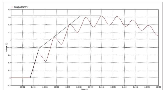
FIG. 5 TRV CHARACTERISTIC DURING SHORT LINE FAULT
