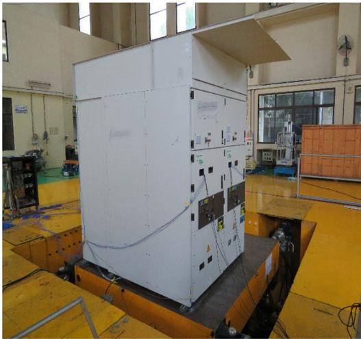
Figure 1. Switchgear unit mounted on shake table.
