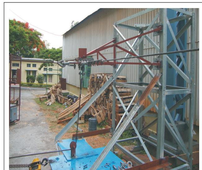
FIG. 4 TEST SET UP FOR 132 kV FRP CROSS ARM
