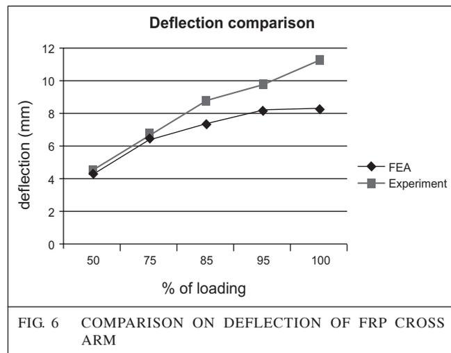
From the above plot, as the intensity of loading increases the deflection in actual testing is slightly more which can be accounted for structural connections and non-linearities present in the FRP cross arm. Further the trend implies that FEA method can be used to analyze the FRP cross arm.
