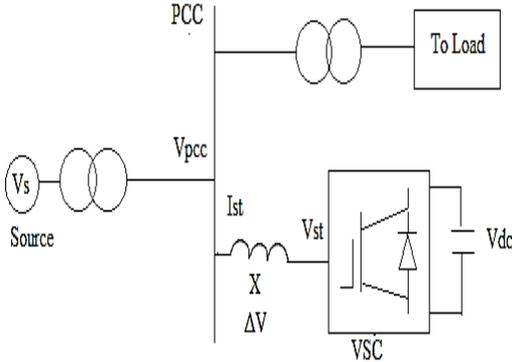
**Figure 2.** Single line diagram of VSC based statcom.
