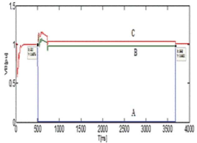
**Figure 6(a).** Voltage variation at BUS B2 during SLG fault at BUS B2.
