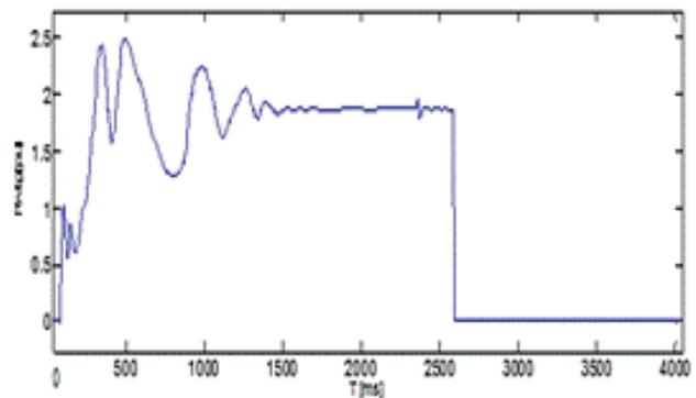
**Figure 6(c).** Power output of wind generator.
