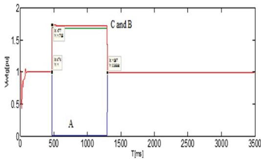
Figure 7(a). Voltage variation during SLG fault at B4 BUS without STATCOM.
