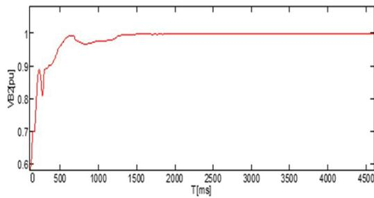
Figure 7(b). Voltage variation during SLG fault at B2 without STATCOM.
