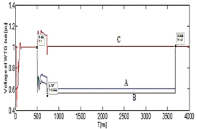
**Figure 6(b).** Voltage variation at BUS B4 during SLG FAULT at BUS B2.
