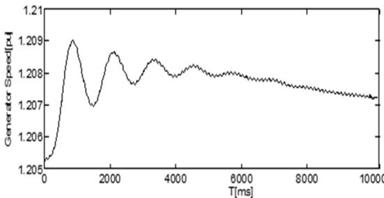
Figure 10(f). Variation of speed of wind generator.
