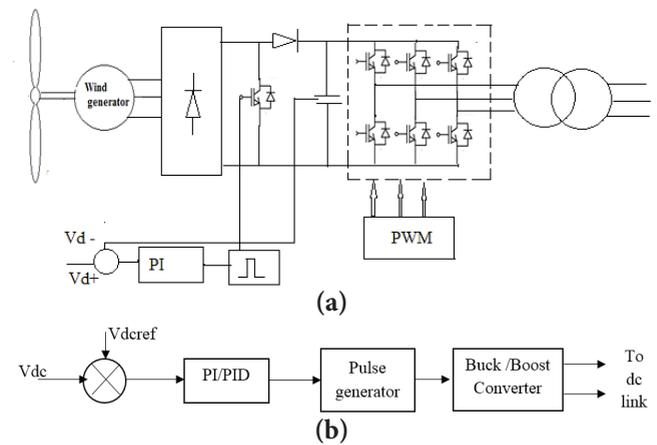
Figure 11. DC link control for wind generator. (a) DC Link Control; (b) Control scheme for dc link
