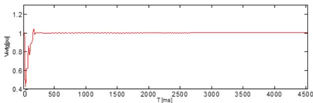
**Figure 6(e).** Correction in voltage at B2 during SLG fault with STATCOM connected at B4.
