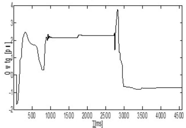
**Figure 12(d).** Variation of reactive power developed by wind generator.
