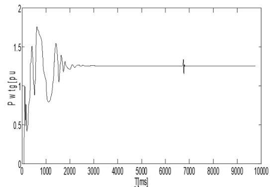
**Figure 6(h).** Power developed by wind generator with active power control action initiated.
