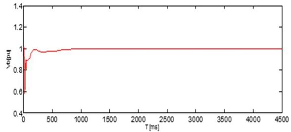
Figure 7(d). FIG. 7(D) Voltage At B2 during Slg fault in presence of Statcom.
