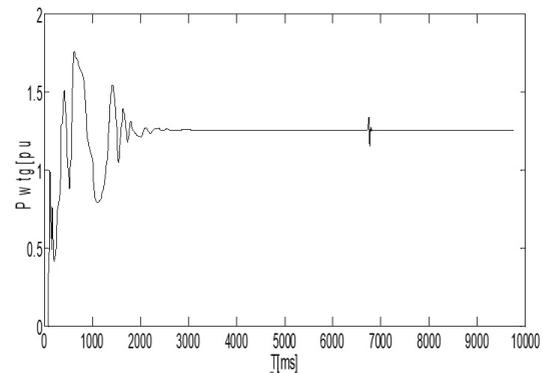
**Figure 6(h).** Power developed by wind generator with active power control action initiated.
