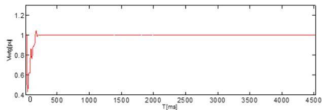
**Figure 6(f).** Correction in voltage at B4 by STATCOM
