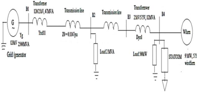
**Figure 5.** Single line diagram of radial transmission network with wind farm.
