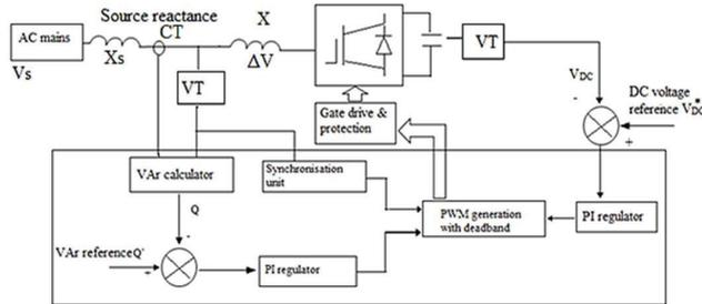
Figure 4. Basic control structure of STATCOM.
