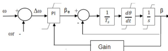
Figure 9. Pitch angle controller for wind generator.
