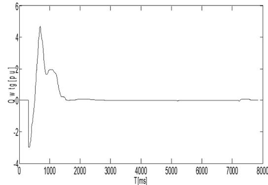
**Figure 6(i).** Reactive power developed by wind generator.
