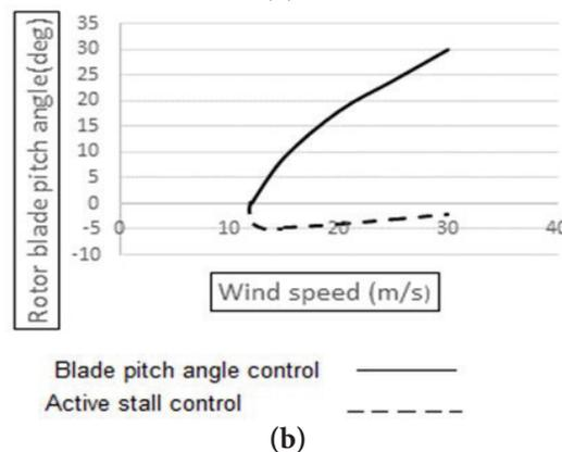
Figure 8. Pitch angle control of wind generator. (a) Pitch angle control of wind generator; (b) Pitch angle( $\beta$ ) Vs wind speed.
