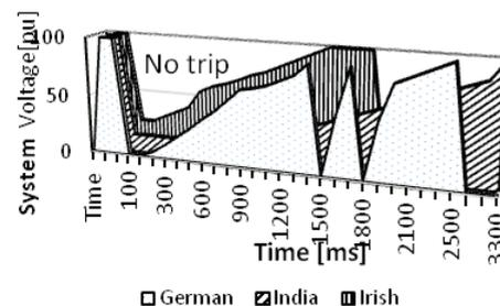
**Figure 1.** Complete fault ride through capability characteristic for German, Indian and Irish systems.
