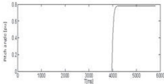
Figure 10(e). Variation of pitch angle of wind generator.
