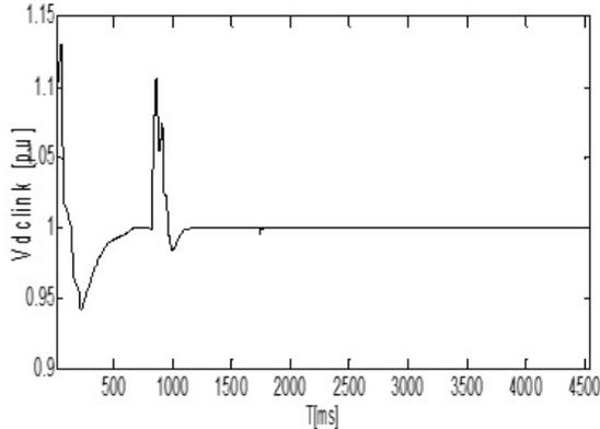
**Figure 12(a).** Variation of DC LINK voltage during fault.
