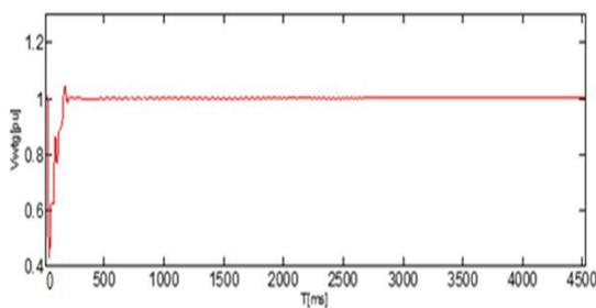
Figure 7(c). Voltage AT B4 BUS during SLG fault in presence of STATCOM.
