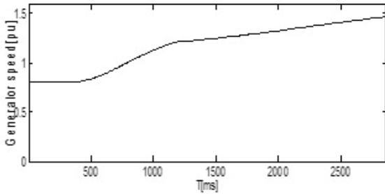
Figure 10(d). Variation of speed of wind generator.
