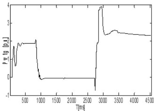
**Figure 12(c).** Variation of active power injected by wind generator at BUS B4.
