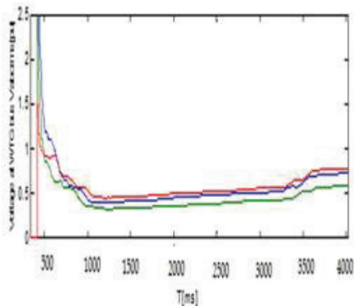
**Figure 12(b).** Variation of voltages at B4 BUS during SLG fault at B4 with DC link control.
