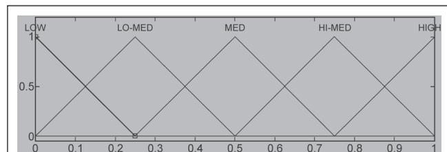
FIG. 5 MEMBERSHIP FUNCTION FOR SENSITIVITY INDEX
