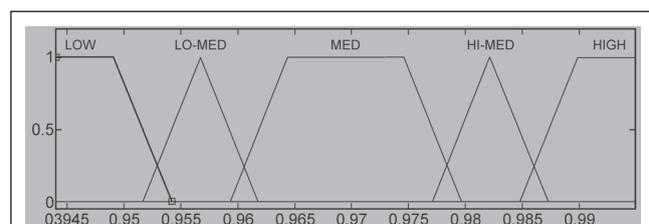
FIG. 4 MEMBERSHIP FUNCTION FOR BUS VOLTAGE
