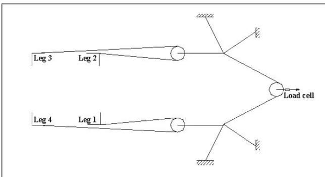
FIG. 6(A) WIND LOAD APPLICATION AT BODY
