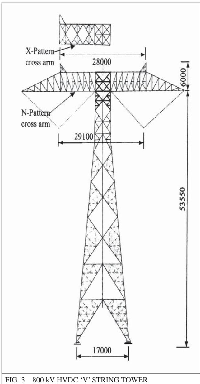
FIG. 3 800 kV HVDC 'V' STRING TOWER
