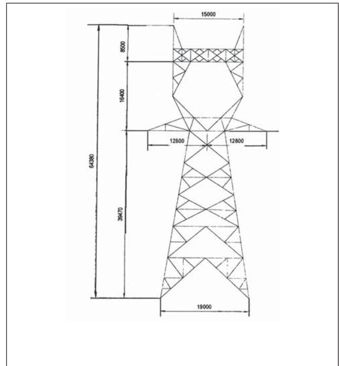
FIG. 1 765 kV S/C TYPE 'C' TOWER
