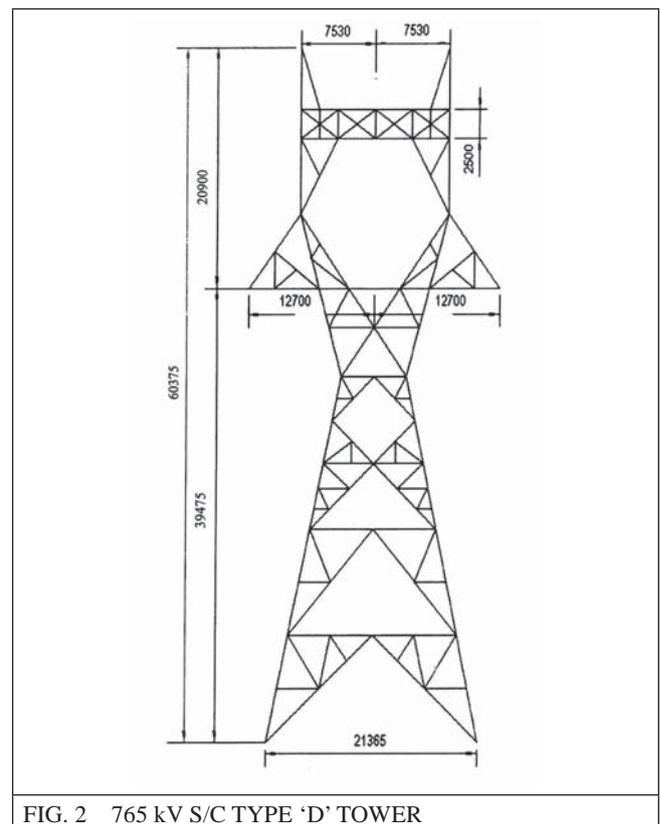
FIG. 2 765 kV S/C TYPE 'D' TOWER
