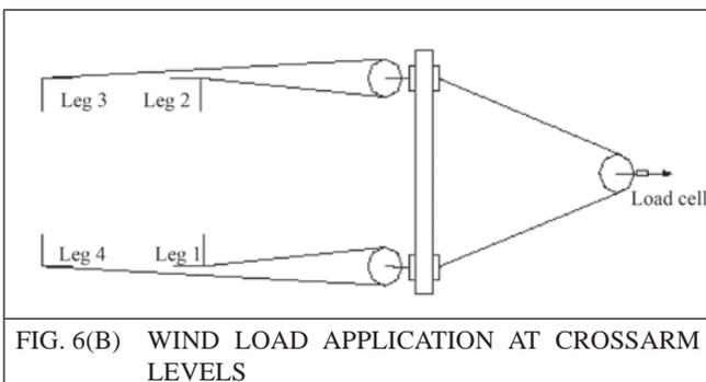
FIG. 6(B) WIND LOAD APPLICATION AT CROSSARM LEVELS
