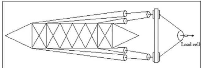
FIG. 6(C) WIND LOAD APPLICATION AT BRIDGE
