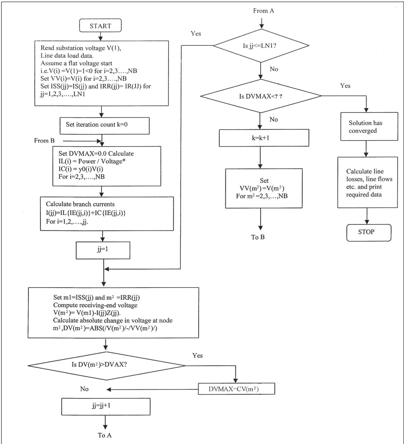
FIG. 4 FLOWCHART FOR LOAD-FLOW CALCULATION OF RADIAL DISTRIBUTION NETWORK
