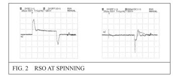
Hence, it was concluded that the rotor was having flying earth fault, and also higher field current indicated inter-turn short during running at rated speed. Rotor was threaded out from the stator bore and for further action, it was sent to the works of the service provider.
