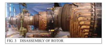
A few slot wedges had shown hair-line cracks of about 10 mm length during DP test. Wedges (both ends) were strengthened with brazing alloy as a preventive action for future. Rotor body was sand-blasted and thereafter, insulating paint was applied on it.
