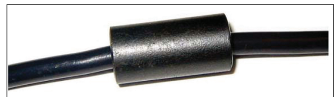
FIG. 9 BASIC CONSTRUCTION OF FERRITE CORE
