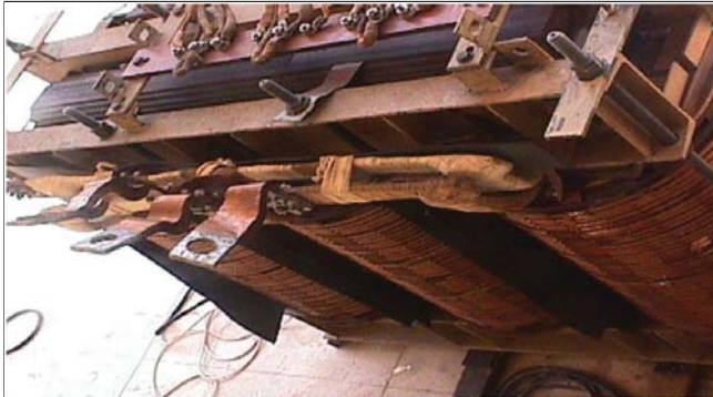
FIG. 1 A VIEW OF THE MODEL TRANSFORMER
