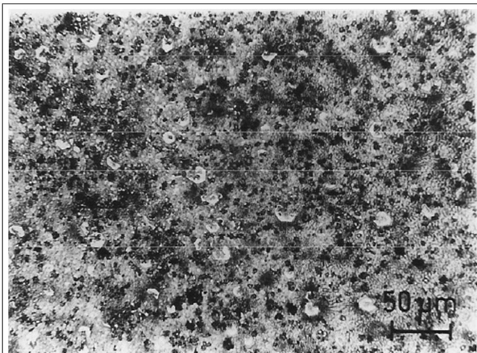
FIG. 1 MICROSTRUCTURE OF 5 % MANGANESE BEARING METAL MOULD HEAT-TREATED (24 mm) SAMPLE
