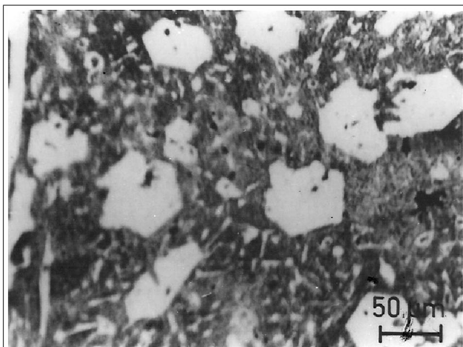
FIG. 2 MICROSTRUCTURE OF 5 % MANGANESE BEARING SAND MOULD HEAT-TREATED (24 mm) SAMPLE
