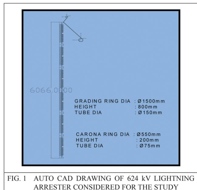
The study of the electrostatic field distribution was conducted with the finite element method. The basic data that was used in the modeling were arrester dimensions, including size and location of ZnO blocks, metal spacers inside the polymer housing, polymer housing geometry and geometry of metal flanges between the
