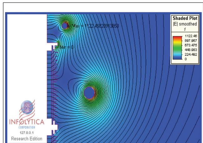
FIG. 3 AN EXPANDED VIEW OF EQUIPOTENTIAL LINES AND SHADED ELECTRIC FIELD DISTRIBUTION OF 624 kV ARRESTER
