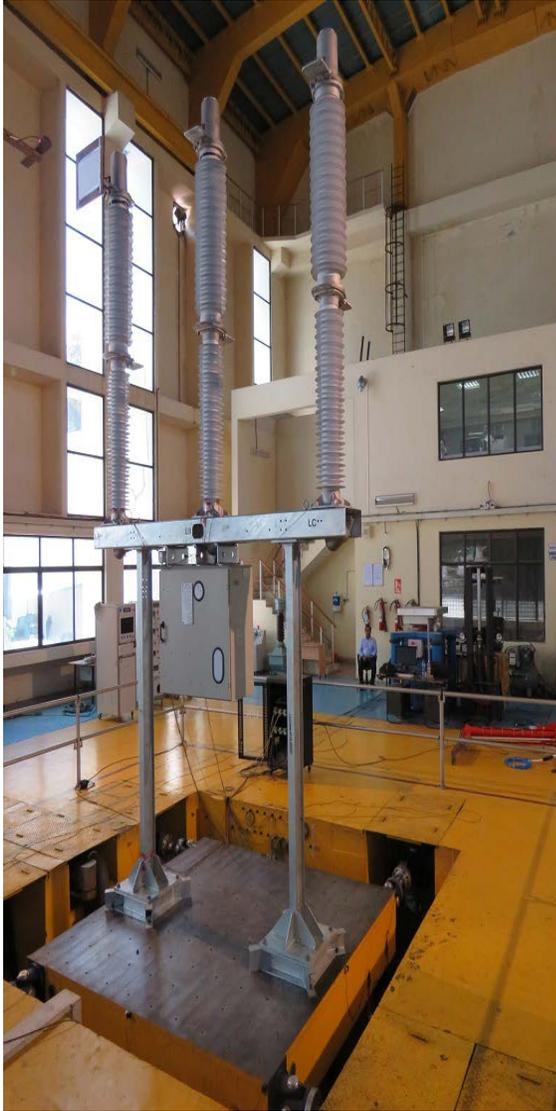
**Figure 1.** 145 kV SF6 circuit breaker mounted on shake table.
