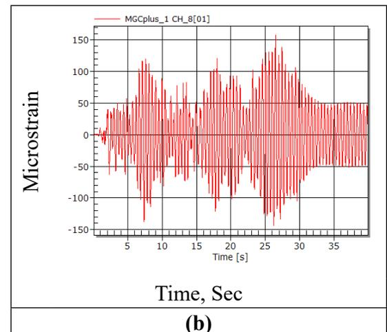
**Figure 6.** (a) Acceleration at common base frame Peak value: +16.28 and -18.10. (b) Time history of strain at bottom of composite insulator on metal end fitting, Peak value = +74.72 and -122.83 microstrain.
