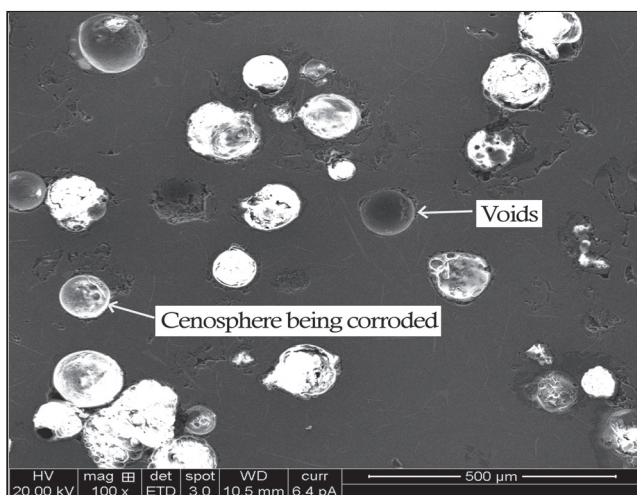
FIG. 4 SEM OF LM6-10% CERAMIC MICROSPHERES COMPOSITES SUBJECTED TO CORROSION (MODIFIED).
