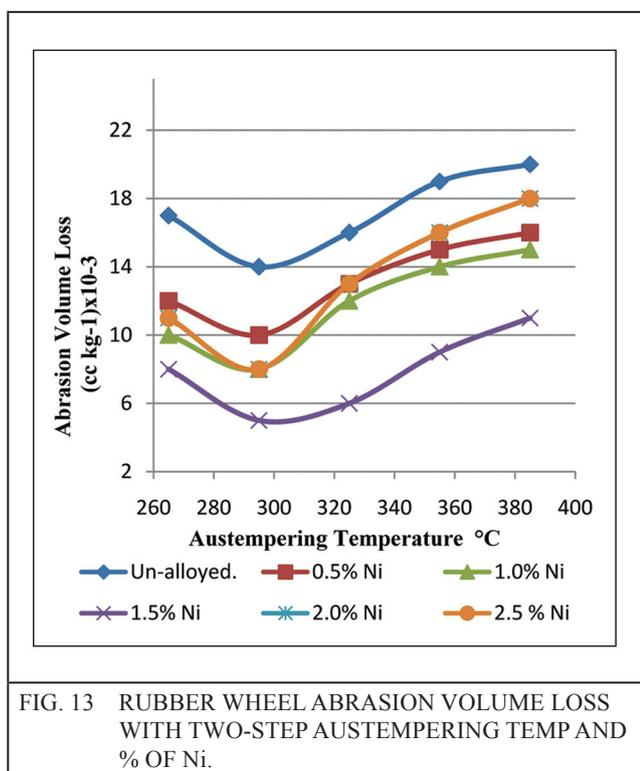
FIG. 13 RUBBER WHEEL ABRASION VOLUME LOSS WITH TWO-STEP AUSTEMPERING TEMP AND % OF Ni.
