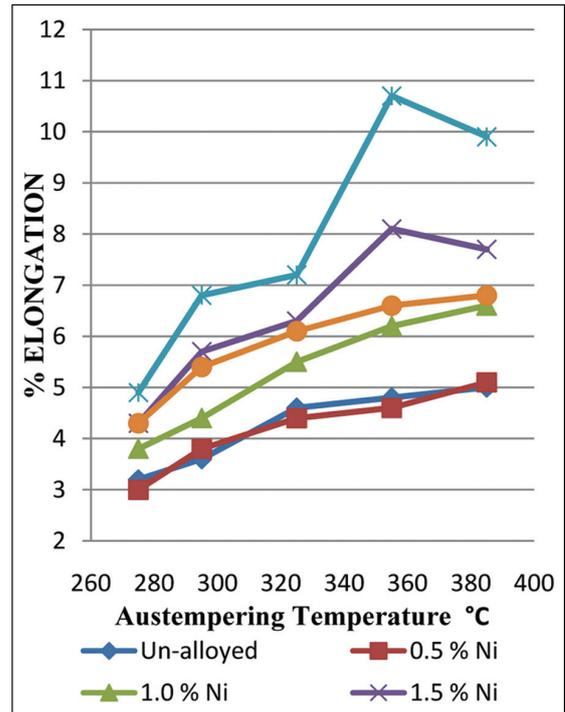
FIG. 11 % ELONGATION VARIATION WITH TWO-AUSTEMPERING TEMP. AND % Ni.
