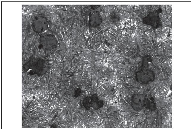
FIG. 6 MICROSTRUCTURE OF PMADI 2.5% Ni SAMPLES AUSTEMPERED AT 340° C (100X-NITAL ETCHED).
